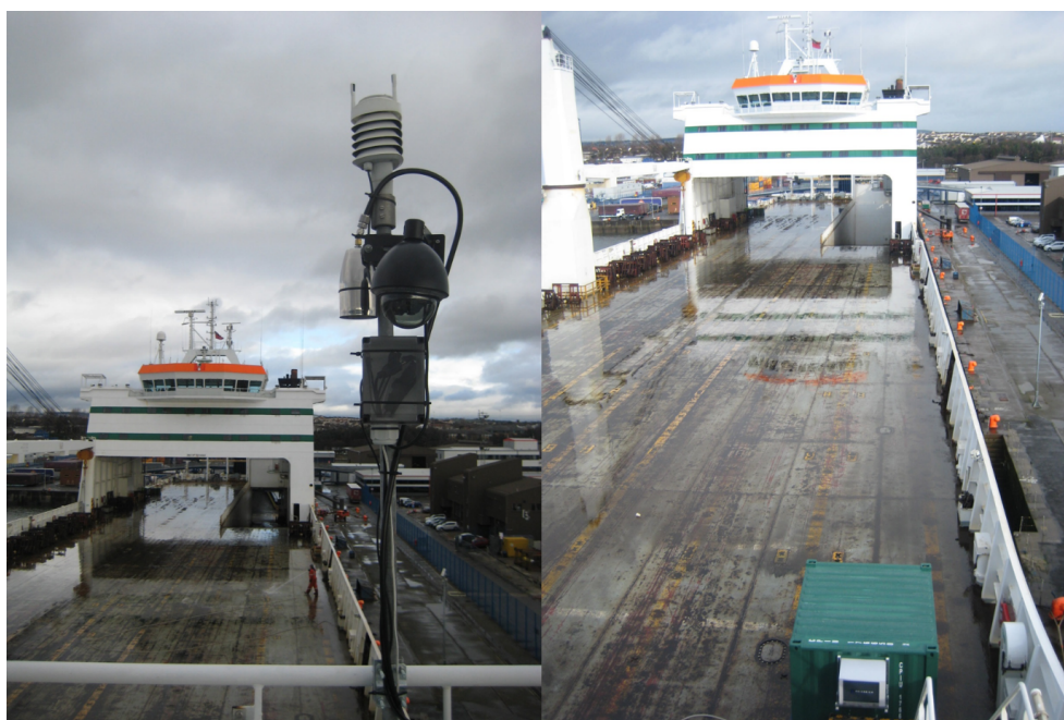
Figure 4. Photos of the North Sea ferry mobile GHG laboratory on the DFDS Seaways Longstone (now the Finnmerchant). View of the (left) weather station mounted on the top deck and (right) from the air inlet mounted on top of the mobile laboratory located on the weather deck.
