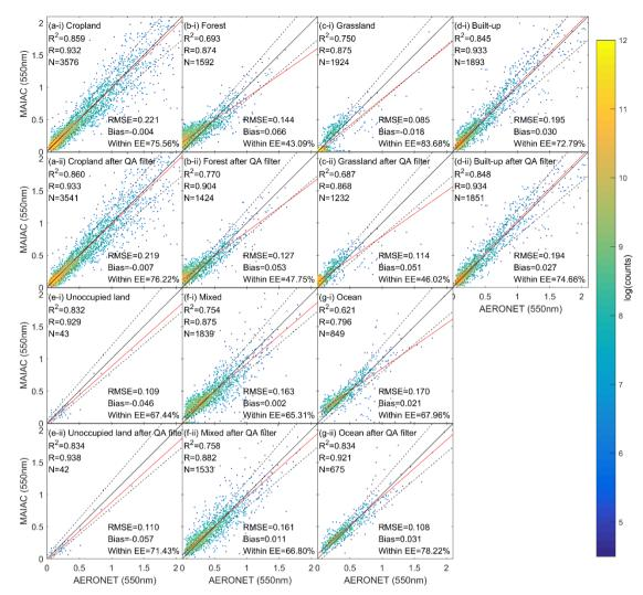
Figure 3. Evaluation of the MAIAC accuracy for different land cover types before and after the QA filter. The black line, red line and dashed line in the scatterplot are the 1:1 reference line, regression line and expected error ( $EE=\pm(0.05+0.15\times AOD)$ ) line, respectively.
