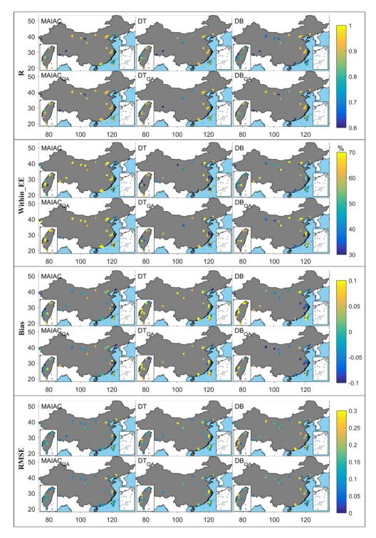
Figure 9. Evaluation results for MAIAC, DT, and DB after and before the QA filter in each AERONET site. The subscript QA denotes the corresponding results after the QA filter.
