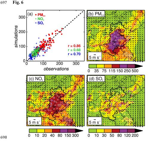
**Figure 6.** The spatial comparisons of predicted and observed episode-average mass concentrations of  $PM_{2.5}$ ,  $NO_2$ , and  $SO_2$ . (a) Statistical comparison of predicted and observed mass concentrations, with the correlation coefficient (*r*). Horizontal distributions of predictions (color contour) and observations (colored circles) of (b)  $PM_{2.5}$ , (c)  $NO_2$ , and (d)  $SO_2$ , along with the simulated wind fields (black arrows).
