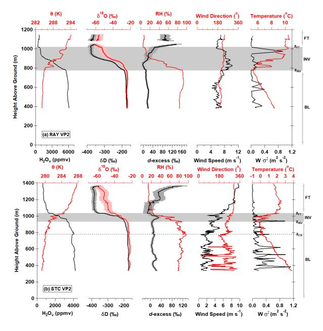
5 Figure 5: Observations of meteorological and isotope variables along the second VP (VP2) conducted on (a) RAY and (b) STC. Measurements in the boundary layer (BL), inversion layer (INV), and free troposphere (FT) are indicated for reference. The dashed grey line in the Fig. 5b corresponds to stratocumulus cloud base (z<sub>CB</sub>).
