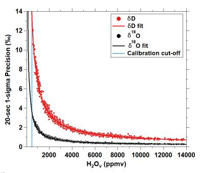
Figure C1: TWVIA  $\delta^{18}$ O and  $\delta$ D 20-s instrument precision (1 $\sigma$ ) as a function of water vapor (H<sub>2</sub>O<sub>x</sub>) mole fraction.
