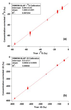
Figure B3. VSMOW-SLAP calibration curves for (a)  $\delta^{18}O$  and (b)  $\delta D$ .  $H_2O_v$ -concentration-corrected isotopic signatures are plotted against the standard's true isotopic signature. Linear regression fit slopes and intercepts are included in the figure insets.
