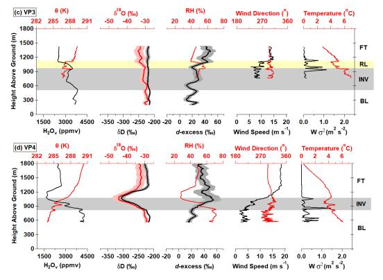
Figure 6: DBL vertical profile (VP) measurements from RF09 in the boundary layer (BL), inversion layer (INV), previous day's residual layer (RL), and free troposphere (FT). Observations corresponding to VP1-4 are shown in (a-d), respectively.
