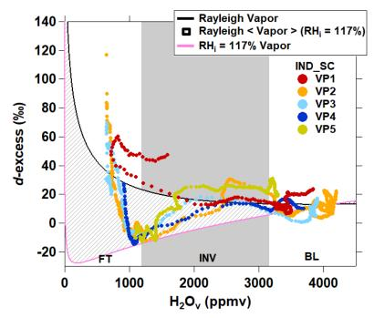
Figure D1: STC VP d-excess observations, Rayleigh vapor d-excess, and calculated d-excess of vapor in ice supersaturated (RHi) conditions up to RHi = 117%. Ice supersaturated conditions were chosen merely to match the INV-FT interface d-excess observations, and do not necessarily reflect a realistic RH<sub>i</sub> for the STC flight day.
