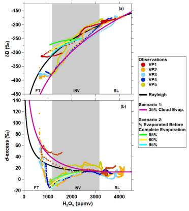
Figure 8: STC vertical profile (VP) (a)  $\delta$ D and (b) d-excess observations plotted with different cloud droplet evaporation scenarios. The two scenarios consider partial cloud droplet evaporation (Scenario 1) or the complete evaporation of previously dehydrated cloud droplets followed by mixing (Scenario 2).
