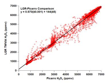
Figure A1: Comparison of calibrated LGR and Picarro  $H_2O_v$  mole fraction measurements from the entire research flight conducted on 6 March 2016 (RAY).
