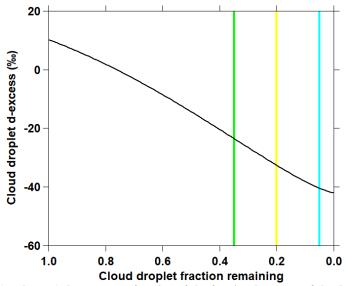
Figure 9. Cloud droplet (condensate) d-excess as a function of the fractional amount of the droplet lost to evaporation (calculated using eqs. 4-6). As cloud droplets dehydrate, d-excess values can become extremely negative. The d-excess signature of cloud droplets that have evaporated by 65%, 80%, and 95% are highlighted. The impact on d-excess of complete evaporation of these previously dehydrated cloud droplets, followed by mixing, is shown in Figure 8.
