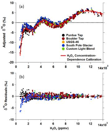
Figure B1: δ<sup>18</sup>O-H<sub>2</sub>O<sub>v</sub> dependence (a) calibration curve and (b) residuals. The true δ<sup>18</sup>O signature of each standard (Table B1) has been subtracted from the TWVIA measurements to give the "adjusted" δ<sup>18</sup>O signature in (a).
