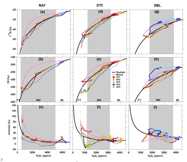
Figure 4: Comparison of vertical profile  $\delta^{18}O$  (top panels),  $\delta D$  (middle panels), and d-excess (bottom panels) measurements to Rayleigh theory (solid) and mixing (pink) curves for three case study days RAY (RF06), STC (RF05), and DBL (RF09). Individual VP descents are indicated by the different-colored points. The average  $H_2O_v$  mole fractions observed within the INV (between  $z_{INV}$  and  $z_{FT}$ ) on each days' VPs are indicated with grey shading.
