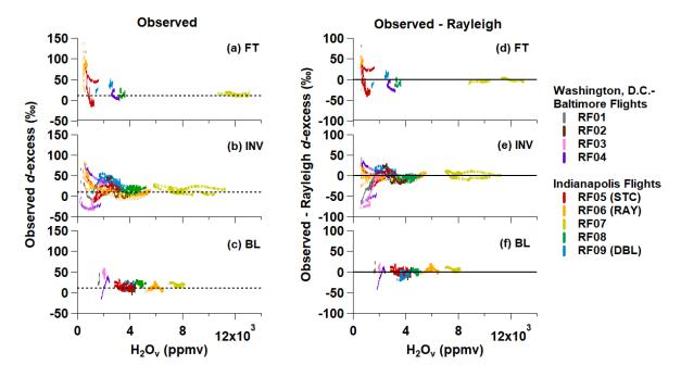
Figure 7: Rayleigh-subtracted d-excess observations in the (a) free troposphere (FT), (b) inversion (INV), and (c) boundary layer (BL) during all the VP descents. Colors indicate each research flight. BL, INV, and FT observations are defined by the rate of change of atmospheric variables, and not defined by  $H_2O_v$  mole fraction.
