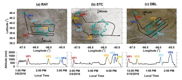
Figure 3: The (a) RAY, (b) STC, and (c) DBL flight path and altitude time series with vertical profiles (VP) highlighted. Flight paths overlay the study site's cloud cover captured at approximately 12:30 local time by the Terra MODIS satellite (https://worldview.earthdata.nasa.gov/). The teal outline indicates the Indianapolis city boundaries. The West Lafayette, IN, Purdue airport is indicated by the airplane marker.
