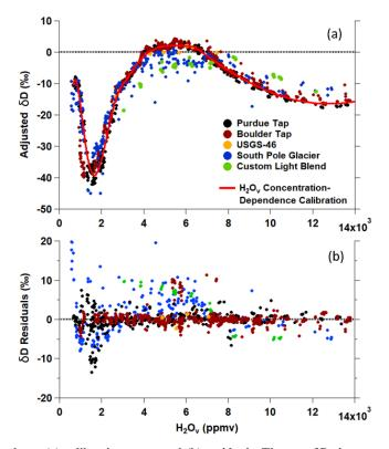
Figure B2: δD-H<sub>2</sub>O<sub>v</sub> dependence (a) calibration curve and (b) residuals. The true δD signature of each standard (Table B1) has been subtracted from the measurements to give the "adjusted" δD signature in (a).
