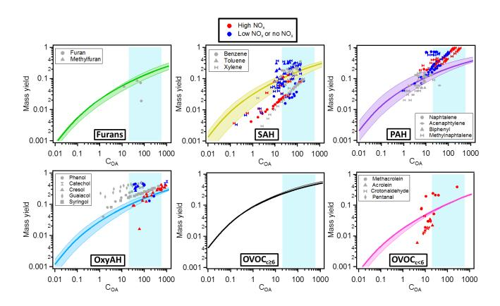
Figure 9. Mass yields for each class of compounds. The solid lines represent the median values while the lower and upper limits are the 25<sup>th</sup> percentile and 75<sup>th</sup> percentiles, respectively. The different markers in each plot are yields published in the literature for
