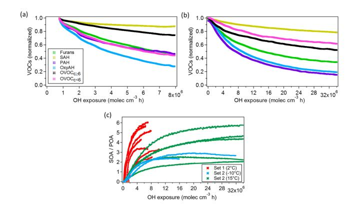
Figure 4. Average consumption of SOA precursor classes against average OH exposure for Set1 (a) and Set2 (b). The observed decay of SOA precursor families (VOCs) as described in Eq. (1) is due to both oxidation processes and dilution in the chamber. c)
