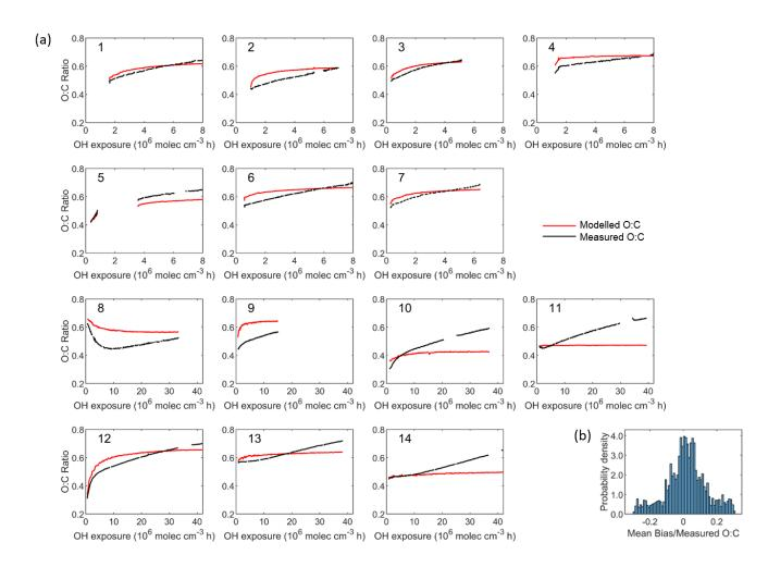
Figure 8. a) Comparison between modelled and measured O:C ratio for each experiment. Set1 (Expt. 1-7, 2°C) and Set2 (Expt. 8-9, -10°C and Expt. 10-14, 15°C). b) Probability distribution of the relative bias (normalized by the averaged measured O:C ratios).
