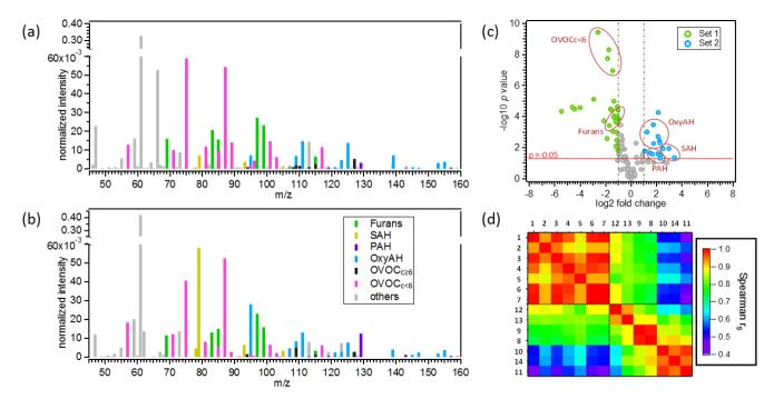
Figure 2. Comparison of the VOC emissions between the two sets of experiments. Panels (a) and (b) display average primary VOCs mass spectra from Set1 (representing the smoldering phase) and Set2 (representing mainly the flaming phase), respectively. Spectra are normalized to the initial total VOC concentration in µg m<sup>-3</sup>. Compounds are color coded by chemical classes. c) *p*-value versus
