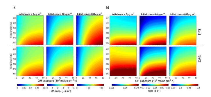
Figure 10. Modelled OA concentrations (a) and yields (b) under different temperature, OH exposure and initial OA concentrations (6, 60 and 600 µg m<sup>-3</sup>). Upper and lower panels are based on Set1 and Set2, respectively. Temperature is provided in Kelvin (K) to avoid confusion with the experimental data in Celsius (°C).
