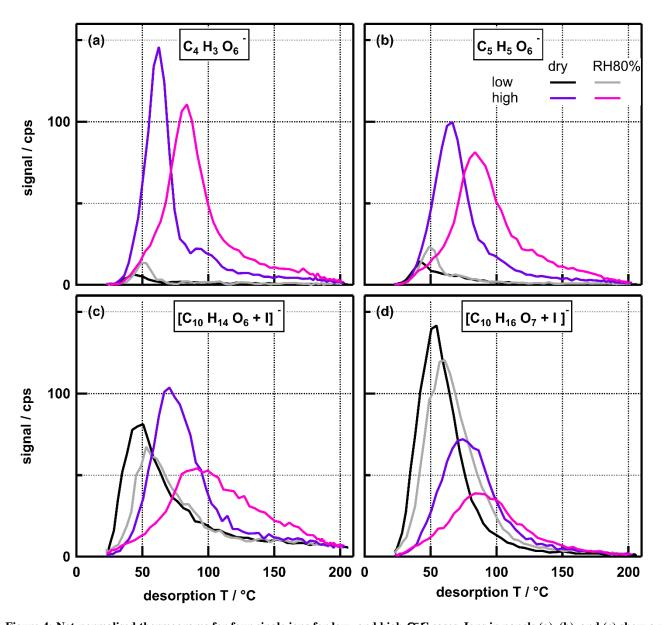
Figure 4: Not-normalised thermograms for four single ions for low- and high-O:C cases. Ions in panels (a), (b), and (c) show a net increase in the RH80% case while the ion in panel (d) had a net decrease in the high-O:C ratio case. Note that the amount of SOA mass collected on the FIGAERO filter was 5-20% higher in the RH80% cases and is also different between the O:C cases.
