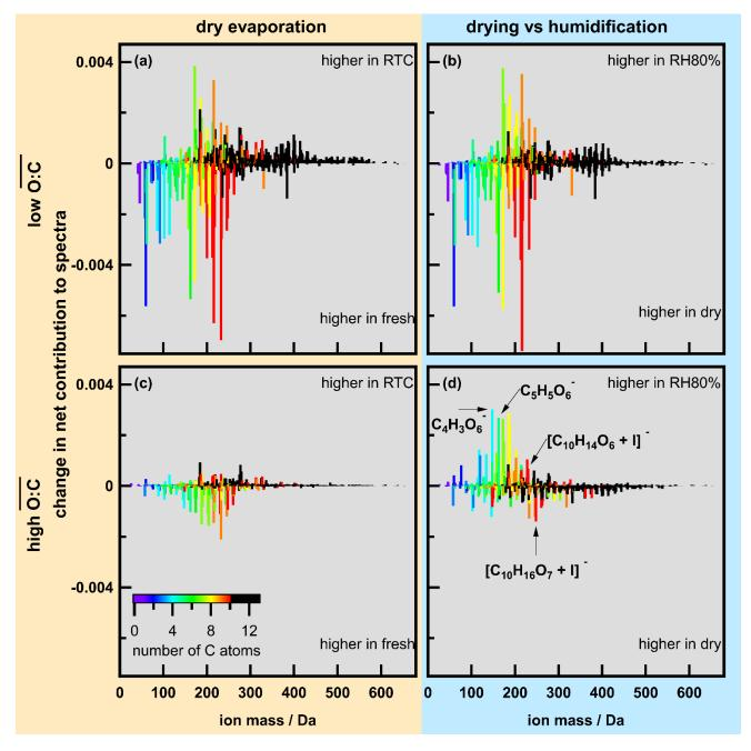
Figure 3: Changes in normalised spectra for low-O:C (top panels: a, b) and high-O:C (bottom panels: c, d). Left column (a, c): changes due to evaporation under dry conditions, right column (b, d): changes between dry and wet conditions. Colour indicates number of C atoms in the identified ions (black corresponds to C-number of larger than 10). Mass spectra were normalised by total signal and then the difference calculated.
