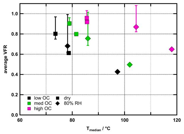
Figure 2: Average VFR during FIGAERO sampling vs median desorption temperature ( $T_{median}$ ) for all experiments. Colours indicate O:C ratios. Measurements under dry conditions are marked with squares, those under RH80% with diamonds. Error bars indicate minimum and maximum VFR observed during sampling time.
