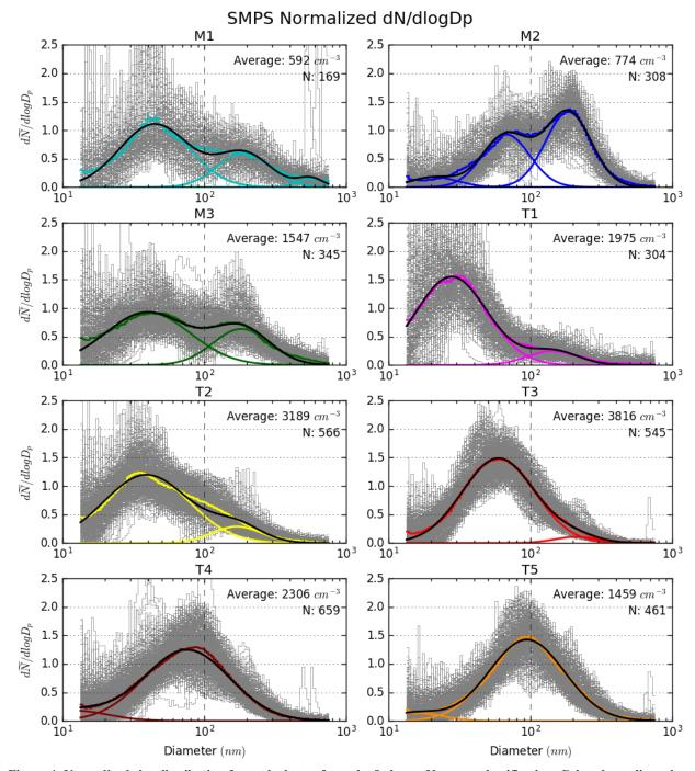
Figure 4 Normalized size distribution for each cluster from the 8 cluster K-means classification. Colored step lines show the average distribution, with best-fit multimodal lognormal fit in black and each mode as colored curves. Observed spectra for each data point in the cluster are shown in grey. Average cluster total particle number concentration and number of data points in each cluster are shown.
