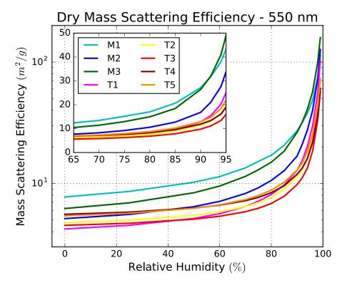
Figure 8 Reconstructed mass scattering efficiencies for each of the cluster population types across a range of environmental relative humidity values. An assumed dry index of refraction of  $1.5 \pm 0.0$  is was used for all population types to highlight the differences in aerosol optical properties expected due to differences in population average size distribution, hygroscopicity, and relative humidity.
