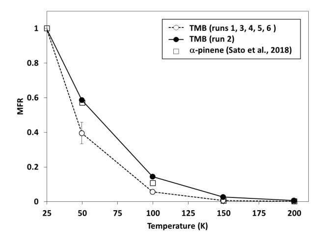
Figure 6. Mass fraction remaining (MFR) for SOA formed from the photooxidation of TMB as a function of thermal denuder temperature (thermogram).
