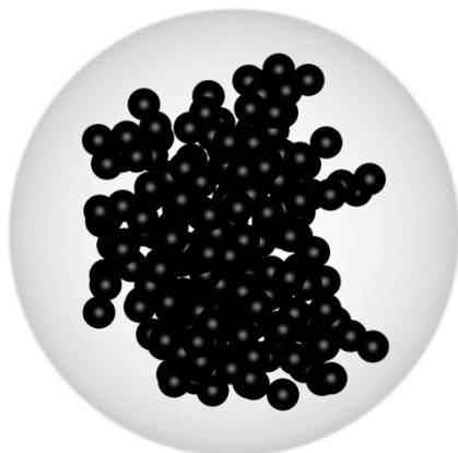
Figure 1: Sketch map of geometry of coated black carbon. An example of fractal black carbon aggregates, containing 200 monomers, is coated by sulfate.
