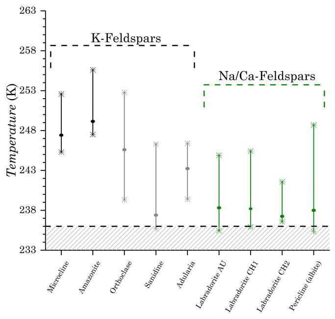
Figure 4. Spread in freezing temperatures corresponding to frozen fraction of 0.1 to 1, for 800 nm feldspar particles. Hashed region indicates homogeneous freezing as the dominant mechansim.
