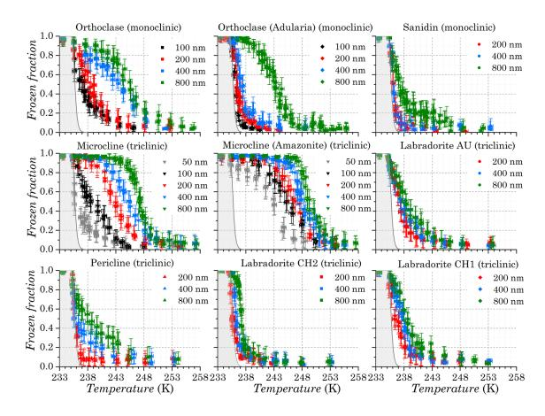
Figure 3. Frozen fractions of size selected feldspar polymorphs. The frozen fraction of water droplets due to homogenous freezing in the setup is given by the grey shaded area. Smaller particles (50 and 100 nm) were only tested for the more ice active samples.
