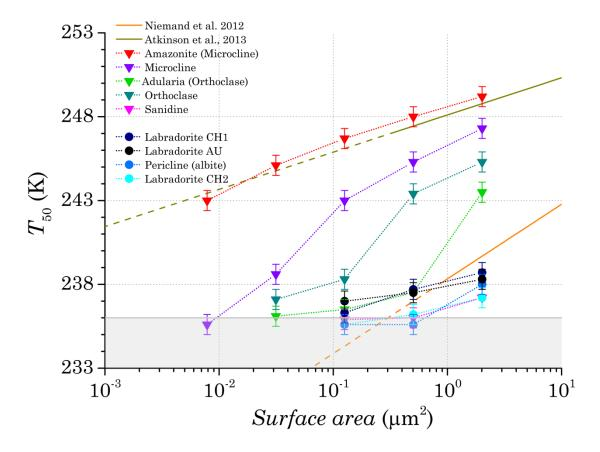
Figure 5. Median freezing temperature ( $T_{50}$ ) where 50% of particles are observed to be frozen as a function of geometric particle surface area. Parameterizations for desert dust from Niemand et al. (2012) and K-feldspar from Atkinson et al. (2013) are included for comparison. Dashed lines indicate extrapolation of the parameterization to lower temperatures.
