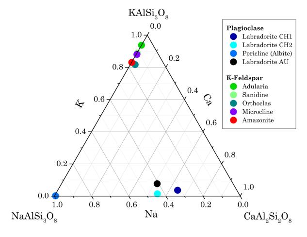
Figure 1. Phase diagram of feldspar samples investigated. Composition determined from X-ray fluorescence spectroscopy (XRF).
