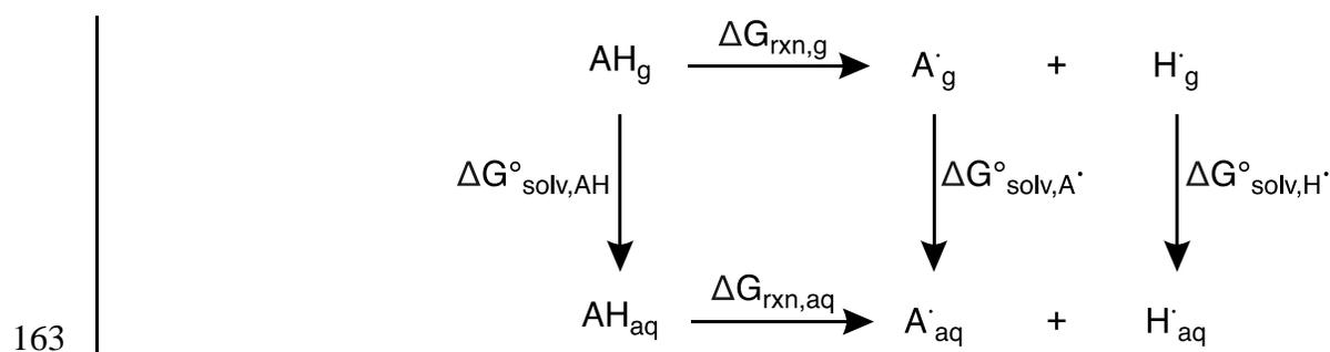
164 **Scheme 1.** Thermodynamic cycle used to calculate bond dissociation free energies.
