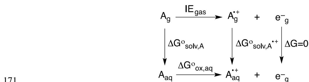
172 **Scheme 2.** Thermodynamic cycle used to calculate oxidation potentials.
