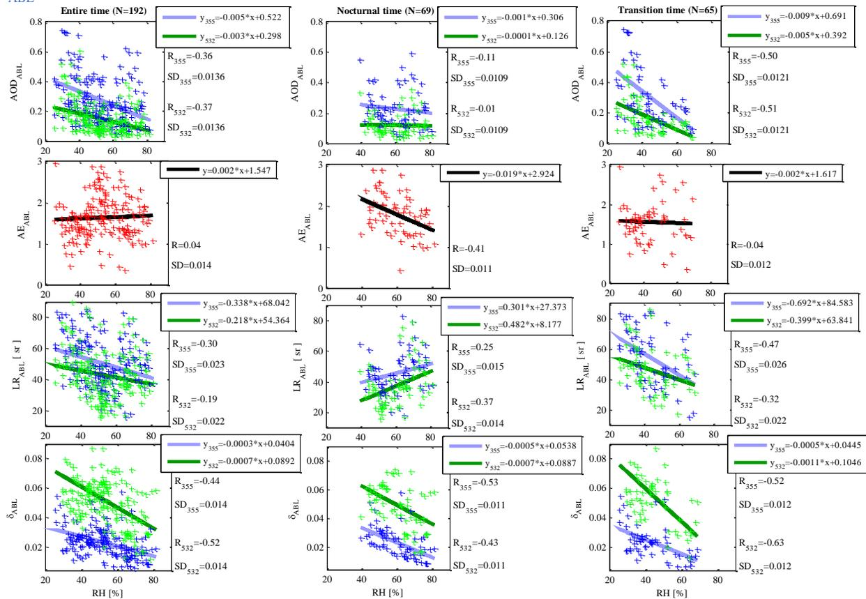
**Figure 2.** Comparison of hourly averaged near-surface relative humidity (RH) measured by the weather transmitter WXT510 (Vaisala) with aerosol optical depth (AOD), Ångström exponent (ÅE), lidar ratio (LR) and particle linear depolarization ratio ( $\delta$ ) derived within boundary layer at 355 and 532 nm from PollyXT lidar at the EARLINET site in Warsaw in period of July-September of 2013, 2015, 2016.
