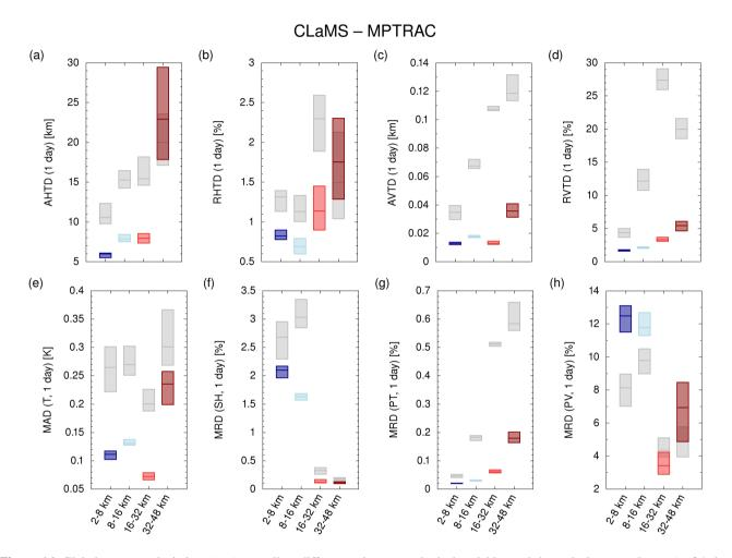
**Figure 16.** Global transport deviations (top) as well as differences in meteorological variables and dynamical tracers (bottom) of 1-day forward trajectories calculated with ERA5 data and the CLaMS or MPTRAC model (blue and red bars). Deviations due to parameterized diffusion and subgrid-scale wind fluctuations imposed on ERA5 trajectories are shown for reference (light gray bars).
