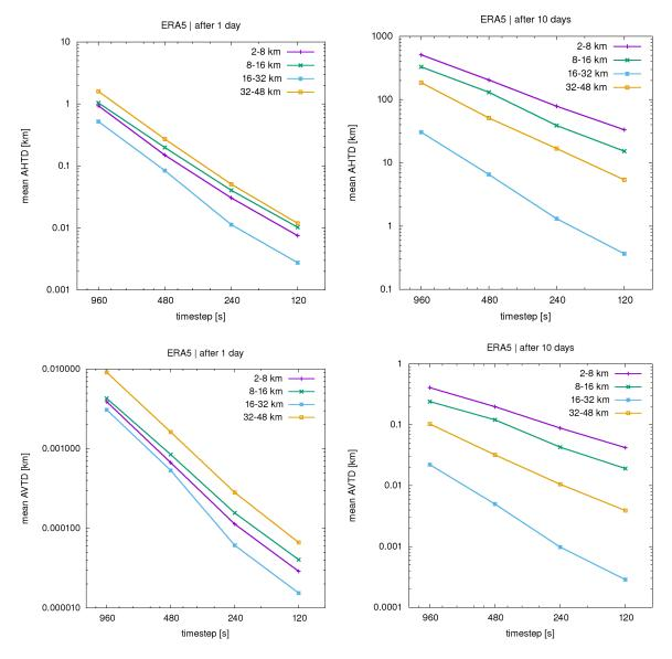
Figure 1: Transport deviations as a function of the time step  $\Delta t$  of the numerical solver used by MPTRAC to calculate ERA5 trajectories.
