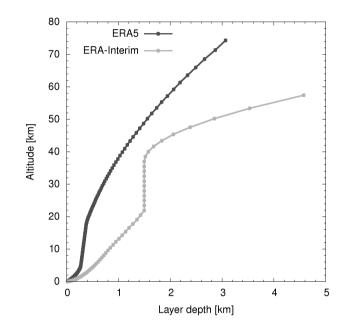
**Figure 1.** Vertical coverage and sampling of the ERA-Interim (light gray) and ERA5 (dark gray) reanalyses. Shown are layer depths and mid-layer altitudes calculated by means of the barometric formula using a constant scale height of 7 km and a surface pressure of 1013.25 hPa.
