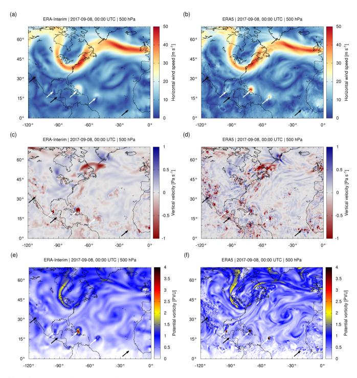
**Figure 2.** Comparison of ERA-Interim (left) and ERA5 (right) horizontal wind speeds (top), vertical velocities (middle), and potential vorticities (bottom) on 8 September 2017, 00:00 UTC over North America and the North Atlantic. Maps refer to the 500 hPa level (about 5 km of altitude). Arrows are used to point out the hurricanes Katia, Irma, and Jose (white, from west to east) as well as examples of gravity waves (gray) and explicitly resolved convective updrafts (black).
