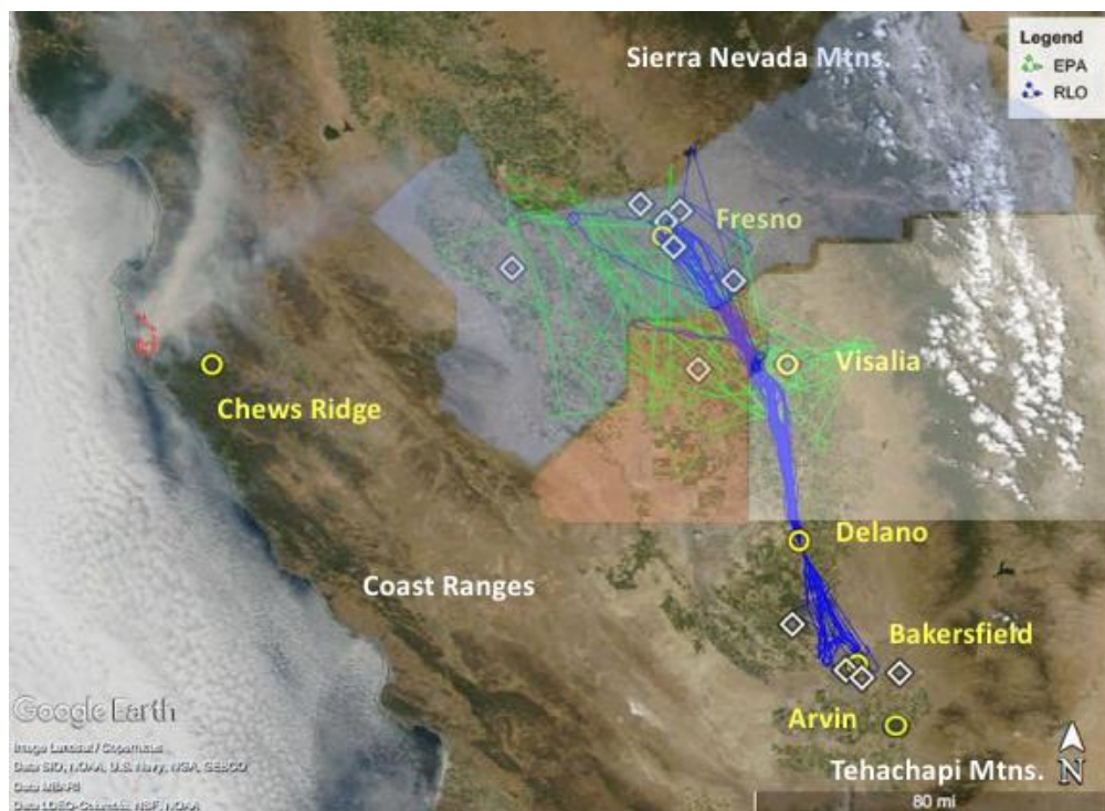
5 Figure 1 Aerial look at the San Joaquin Valley. Yellow circles are important sites which are labelled. The green lines are flight tracks from the EPA flights and the blue are from the RLO flights. White diamonds are CARB surface stations. Active fires on the ground can be seen as small red outlines to the Northwest of the Chews Ridge site (available at: https://worldview.earthdata.nasa.gov/ , 2018a) from July 27, 2016. Major mountain ranges are labelled in white. The three shaded regions are at top in blue is Fresno County, bottom left in red is Kings County, and bottom right in white is Tulare County.
