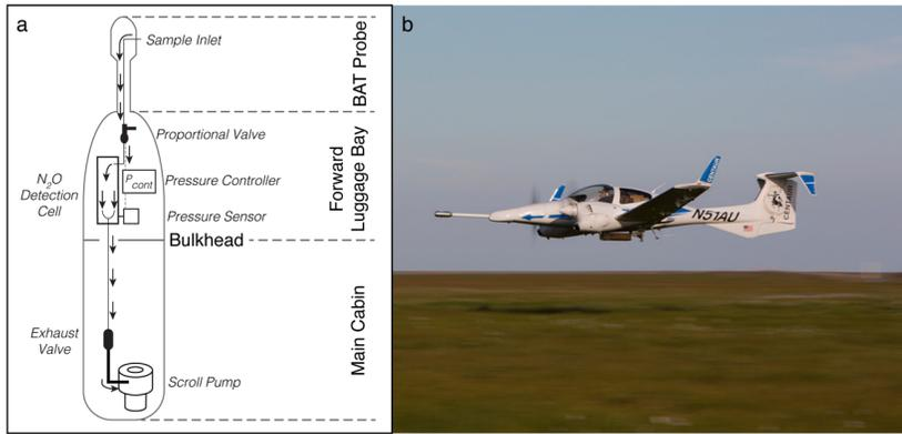
**Figure 1.** FOCAL during flight. **a.** Top-down schematic of the atmospheric gas flow through the aircraft (not to scale). The sample inlet is located on the BAT probe, located at the nose of the plane. The gas is pumped through the pressure-regulated detection cell of the ICOS spectrometer, located within the luggage bay in front of the pilot. **b.** Image of the Diamond DA-42 flying around 15 m above the surface.
