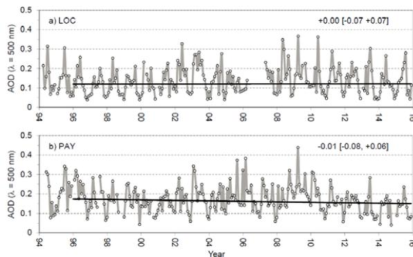
Figure 3: Time series of monthly AOD ( $\lambda = 500$  nm) averages available since 1994 at: a) LOC and b) PAY. The 1996 – 2015 decadal trend is shown in the top right-hand corner where values in brackets represent the upper and lower bounds of the 90% confidence interval. Trend values are only shown for the 1996 – 2015 period to be consistent with other trend periods in this study.
