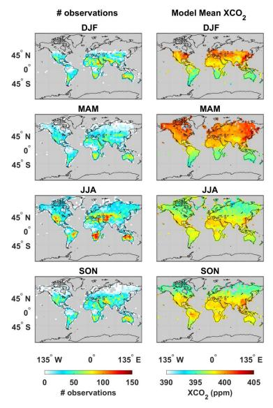
$Figure~2:~Total~number~of~OCO-2~LN~and~LG~XCO_2~observations~(left~column)~and~the~corresponding~seasonally-averaged~multi-model~(NASA-CASA, CASA-GFED, SiB-4~and~LPJ~biosphere~models)~mean~GEOS-Chem-simulated~prior~XCO_2~(ppm)~(right~column)~in~2015.$
