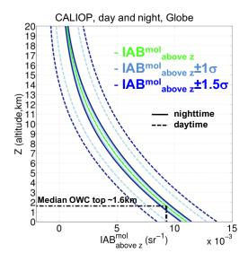
**Figure B1:** Nighttime (solid) and daytime (dashed) simulated vertical profile of integrated attenuated backscatter above any given altitude, z, IAB<sup>mol</sup><sub>above z</sub> (green curve). The light blue (respectively dark 68
