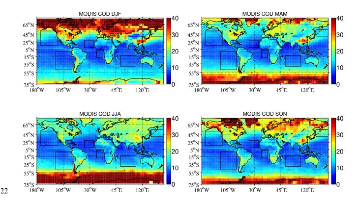
Figure A2: Seasonal maps of COD used in the calculations of DARE<sub>OWC</sub>. COD information is inferred from MODIS seasonally averaged monthly 1°x1° grids (i.e. liquid water cloud products of MYD08\_M3: "Cloud Effective Radius Liquid Mean Mean" and "Cloud Optical Thickness Liquid Mean Mean" [Platnick et al. 2015]) from 2008 to 2012. The squares show different regions defined in Table 6.
