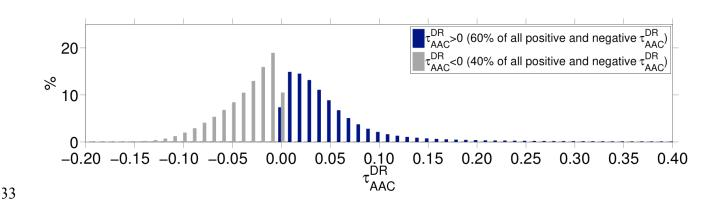
Figure 3: Global distribution of  $\tau^{DR}_{AAC}$  at 532 nm. Positive (i.e., valid)  $\tau^{DR}_{AAC}$  values are in dark blue (N~3.4M) and negative  $\tau^{DR}_{AAC}$  values in grey (N~2.2M). These are nighttime CALIOP measurements from 2008-2012.
