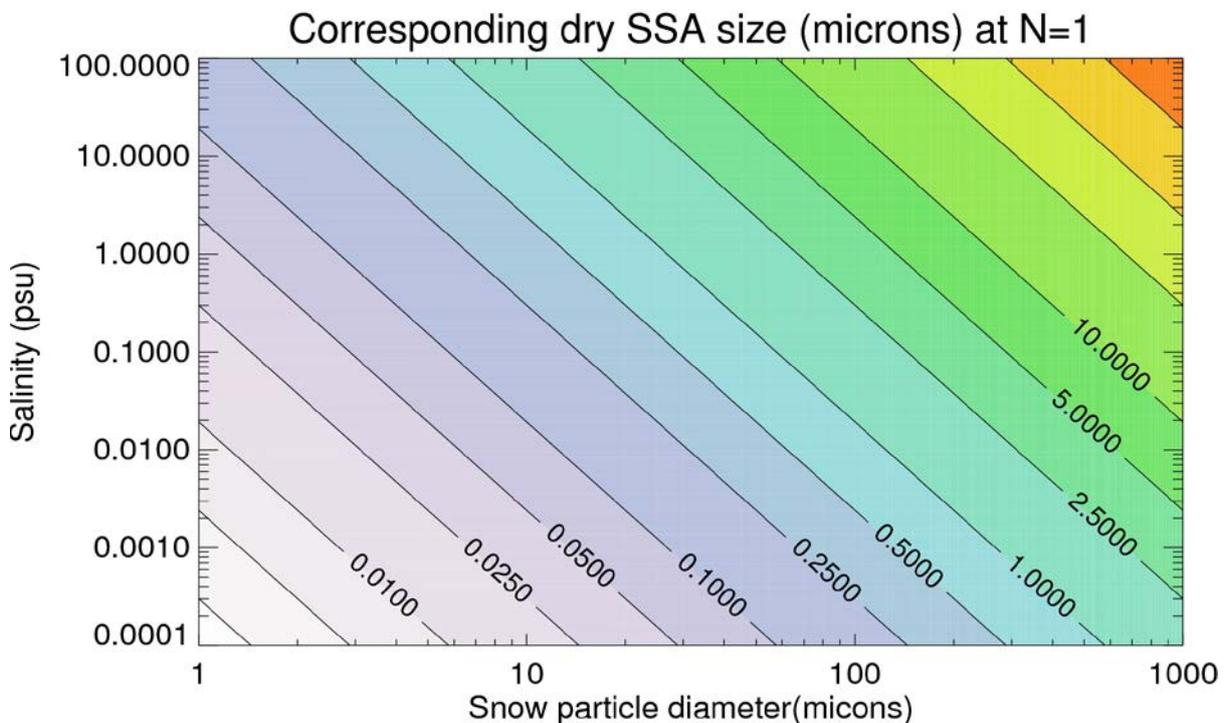
Figure: Equivalent dry SSA diameter ( $\mu\text{m}$ ) as a function of initial snow particle diameter ( $\mu\text{m}$ ) and snow salinity (psu) for N=1, calculated following equation 11.
