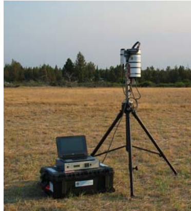
Fig. 2. Setup of the GUVis-3511 radiometer at Smith Rock State Park. The radiometer (white cylinder), BioSHADE assembly and BioGPS are mounted on a tripod. Shown next to the instrument is the laptop for recording the data, the instrument's control unit, and a black case containing the power source.
