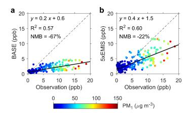
Figure 4. Comparison of modeled and observed HCHO concentrations. (a) BASE scenario. (b)  $5 \times \text{EMIS}$  scenario. The dots are colored according to PM<sub>1</sub> concentrations. Model results from WRF-Chem are shown.
