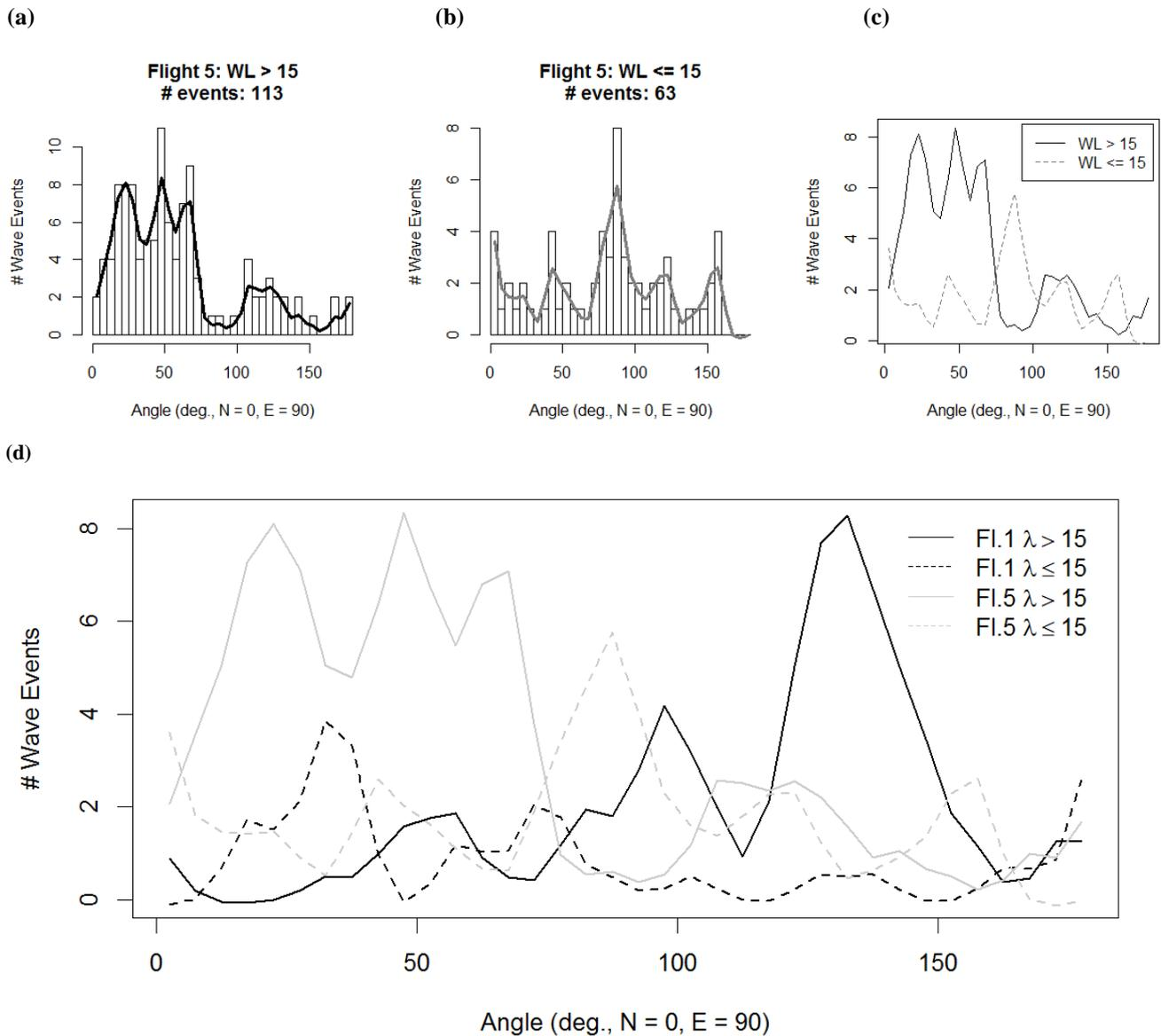
Figure 12 same as Figure 9 but for flight 5. In this case, the results for both wavelength ranges are qualitatively stable for different  $n$  and  $t$  (the smaller  $n$  and  $t$ , the higher the absolute values). Part (d) shows the direct comparison of the results of both flights.
