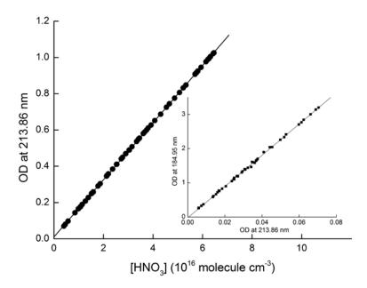
**Figure 2**: Beer-Lambert plot used for the calculation of the HNO<sub>3</sub> absorption cross section at 213.86 nm,  $\sigma_{213.86 \text{ nm}}$ . The inset shows the linear relation between optical densities (OD) at 184.95 nm and 213.86 nm.
