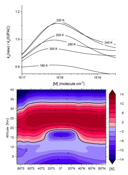
**Figure 11**. Upper panel: Ratio of rate coefficients obtained by combining results from this work with selected datasets from the literature,  $k_5$ (new), to those presently recommended by IUPAC,  $k_5$ (IUPAC). Lower panel: percentage change in rate coefficient  $k_5$  calculated using annually and zonally averaged temperatures and pressure in the EMAC model.
