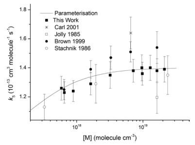
**Figure 9.** Comparison of room temperature rate coefficients ( $k_5$ ) obtained in nitrogen bath gas. The error bars on our data points represent total uncertainty. The solid line are values of  $k_5$  at 297 K from the parametrization obtained by fitting to the temperature and pressure dependent datasets from Brown et al. (1999), Stachnik et al. (1986), and this work.
