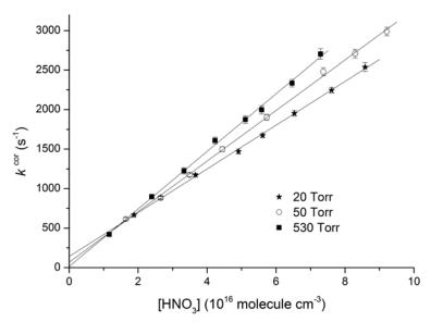
**Figure 6**. Corrected pseudo-first-order rate coefficients,  $k^{\text{cor}}$ , plotted as a function of the HNO<sub>3</sub> concentration. The data were obtained at 242 K and at three different pressures.
