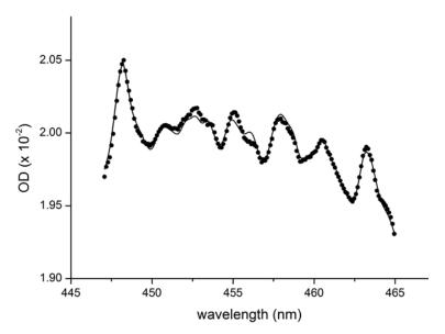
**Figure 4.**  $NO_2$  impurity measurement (experiment at 298 K, 18 Torr) using the ternary mixture. The dotted line is the experimental  $NO_2$  optical density (OD); the solid line is the fitted optical density using a reference spectrum (Bogumil et al., 2003). In this measurement, the  $NO_2$  impurity corresponded to 0.01% of the  $HNO_3$  concentration.
