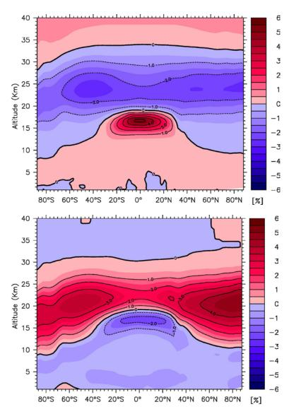
**Figure 12.** Impact of the results from this work in a global atmospheric chemistry model (EMAC). The contours indicate the percentage change in the predicted mixing ratios (zonal and annual average) of  $HNO_3$  (upper panel) and NOx (lower panel), which result from the new parameterization of  $k_5$ .
