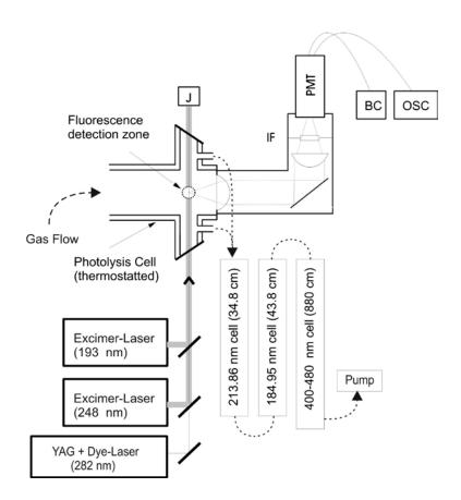
**Figure 1:** PLP-LIF setup. MFC = mass flow controller, PMT = photomultiplier tube, J = Joule meter, BC = box-car data acquisition, OSC = oscilloscope, IF = interference filter (309  $\pm$  5 nm). Capacitance manometers monitored the pressure inside the reactor and the three optical absorption cells.
