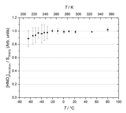
**Figure 3.** TPEFS detection of  $HNO_3$  in the center of the reactor at different temperatures. The TPEFS signal ( $S_{TPEFS}$ ) has been normalised to the  $HNO_3$  concentration. The error bars indicate uncertainty derived from correction to the TPEFS signal due to quenching of fluorescence and absorption by  $HNO_3$ .
