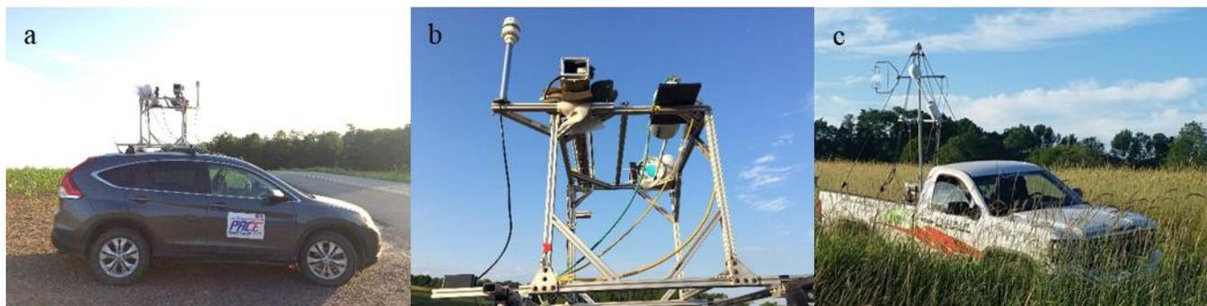
Figure 1. (a) The Princeton atmospheric chemistry experiment (PACE), (b) close-up of PACE roof rack with
