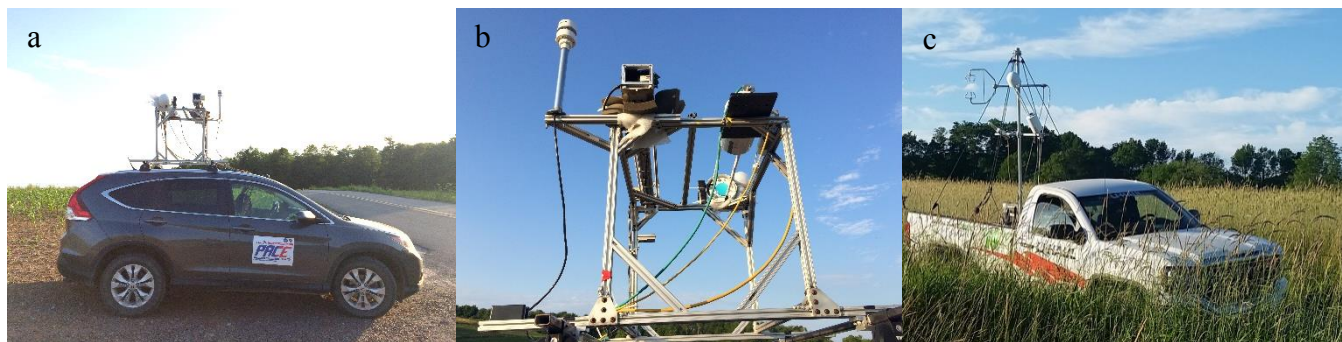
Figure 1. (a) The Princeton atmospheric chemistry experiment (PACE), (b) close-up of PACE roof rack with instrumentation and (c) mobile tower platform.
