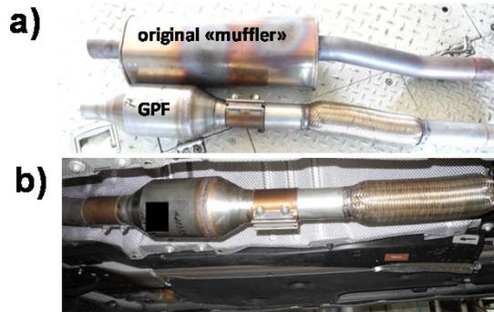
Figure S12. Pictures of a) original “muffler” and GPF in comparison, b) retrofitted GPF, installed underfloor in replacement to “muffler”.
