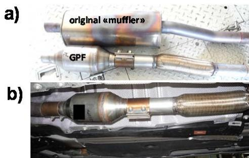
**Figure R2-1:** “Pictures of **a)** original “muffler” and GPF in comparison, **b)** retrofitted GPF, installed underfloor in replacement to “muffler”.”
