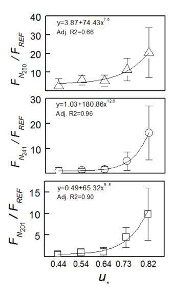
Figure 5. Dust emission ratio dependencies on friction velocity and livestock density. Open triangles ( $\triangle$ ), circles ( $\circ$ ), and squares ( $\square$ ) denote dust emission values from the trampled surfaces with livestock densities of 250, 241, 201 Headha<sup>-1</sup>, respectively. a) Relationships between the mean emission ratio (of  $F_N/F_{REF}$ ) and  $u_*$  for N of 201, 241and 250 Headha<sup>-1</sup>;  $b_*$ .
