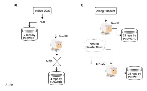
Figure 3. A schematic flowchart of PI-SWERL<sup>®</sup> experimental test a) for zero and trampling of  $N_{250}$  inside DOS; and b) for trampling of  $N_{201}$  and  $N_{241}$  along transect areas. PI-SWERL<sup>®</sup> experimental replications for each dataset is marked as *reps*.
