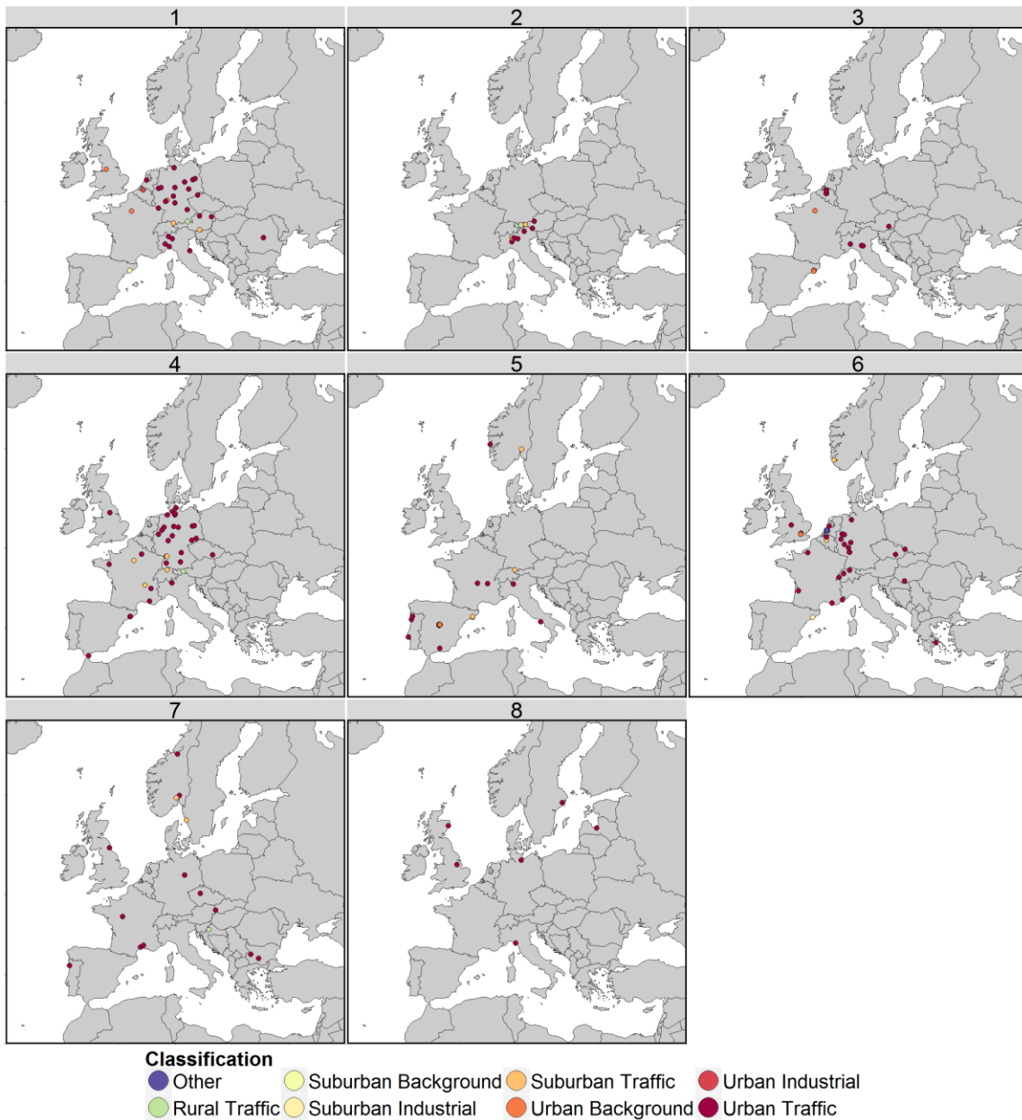
Figure S11: Map of sites with 2010-2014 annual \text{NO}_2 concentrations ( \text{NO}_{2\text{AA}} ) between 40\text{-}50 \mu\text{g m}^{-3} , grouped into clusters demarcating distinct variations in monthly, hour of day, and hourly \text{NO}_2 concentration bin contributions to 2010-2014 \text{NO}_{2\text{AA}} .
