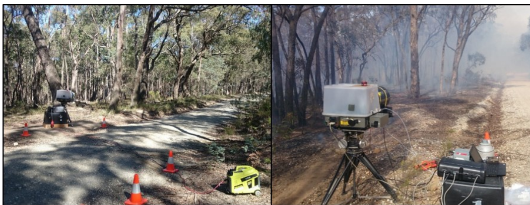
Figure 2. The instrumental set-up for the open-path FTIR measurements of smoke at Greendale on April 13 th , 2015 (left) and Castlemaine on April 23 rd , 2015 (right).
