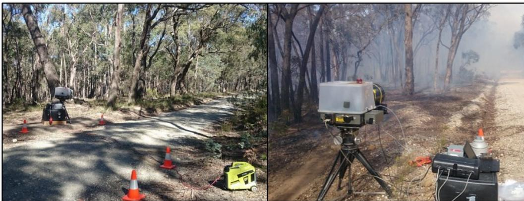
**Figure 2.** The instrumental set-up for the open-path FTIR measurements of smoke at Greendale on April 13<sup>th</sup>, 2015 (left) and Castlemaine on April 23<sup>rd</sup>, 2015 (right).
