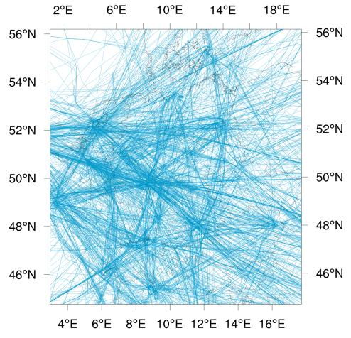
Figure 2. Flight trajectories for the COSMO-DE domain derived from ADS-B data (08 UTC - 16 UTC 3 December 2013). Each trajectory is plotted as a faint dashed line. Seemingly solid or thick lines are indicative of multiple overlaid trajectories.
