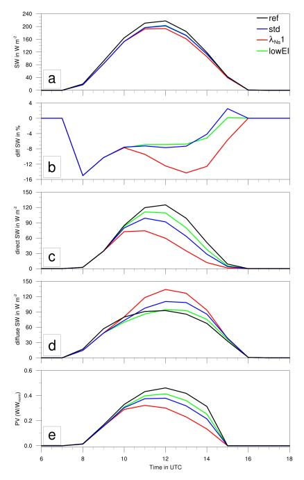
**Figure 12.** Temporal evolution for 3 December 2013 of incoming shortwave radiation: reference (black); aviation simulation as before (blue); "bio-fuel" scenario with  $EI_{iceno} \times 0.1$  (green), omission of crystal loss during contrail vortex phase with  $\lambda_{Ns} = 1$  (red): a) total; b) difference in total SW between aviation simulation and reference simulation c) direct; d) diffuse; e) normalized PV-power diffuse; all for the location marked with the red circle in Fig. 11.
