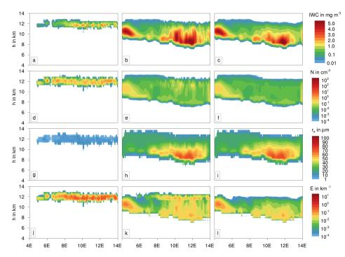
**Figure 6.** Vertical cross section of various contrail properties at 12 UTC along the black line in Fig. 4: ice water content, ice crystal number concentration, effective radius, and extinction coefficient (from top to bottom). Depicted are the simulation with aviation (left column: contrail class; middle column: cirrus cloud class) and without aviation (right column).
