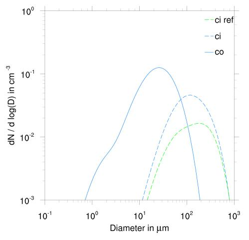
Figure 1. Ice crystal size distribution of the simulation with (blue) and without (green) aviation. For the simulation with aviation, separate ASDs of the contrail and cirrus cloud class are shown (solid and dotted line). 12 UTC.
