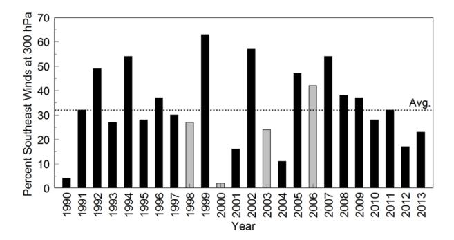
Figure 2. Percent of 300 hPa wind directions between 67.5° and 202.5° for each year 1990 to 2010 for mid-November through December. Experiment years are shaded gray. The average over 20 years is shown by the dashed line.
