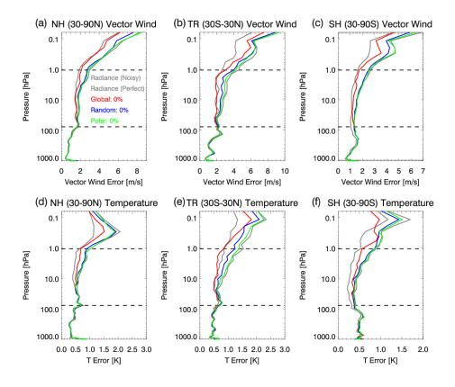
**Fig. 16.** RMS vector wind errors on 1 December 2014 for (a) NH, (b) TR, and (c) SH and RMS temperature errors for the (d) NH, (e) TR, and (f) SH. Colored lines are for ozone assimilation experiments with noisy radiance and perfect ozone data using
