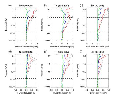
**Fig. 17.** RMS vector wind error differences (with respect to assimilation of radiance only) on 1 December 2014 for (a) NH, (b) TR, and (c) SH and RMS temperature error differences for the (d) NH, (e) TR, and (f) SH. Lines are for ozone assimilation
