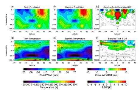
Fig. 5. Zonal mean zonal wind for the (a) truth experiment and (b) baseline experiments and (c) baseline-truth zonal wind difference. Zonal mean temperature for the (d) truth experiment and (e) baseline experiment and (f) baseline-truth temperature
