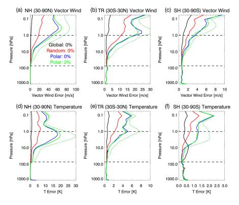
Fig. 13. RMS vector wind errors on 1 December 2014 for (a) NH, (b) TR, and (c) SH and RMS temperature errors for the (d) NH, (e) TR, and (f) SH. Solid (dotted) lines are for ozone assimilation experiments (baselines) for global: 0% error (black),
