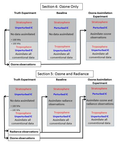
**Fig. 4.** Schematic diagram to illustrate the design for the experiments analyzed in Sect. 4 and Sect. 5. The truth experiment (TE) in both cases assimilates all conventional data in the troposphere (pressures < 100 hPa) and no data in the stratosphere (pressures < 100 hPa). In Sect. 4, the baseline experiment is the same as the TE, except for perturbed initial conditions (IC)
