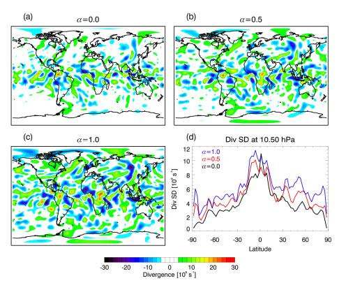
Fig. 11. Horizontal maps at 10.5 hPa of the divergence on 1 December 2014 for ozone assimilation experiments with (a)  $\alpha = 0.0$ , (b)  $\alpha = 0.5$ , and (c)  $\alpha = 1.0$ . Colors show divergence with red (blue) indicating high (low) values. (d) The standard deviation of the divergence as a function of latitude at 10.5 hPa. Lines are  $\alpha = 0.0$  (black),  $\alpha = 0.5$  (red), and  $\alpha = 1.0$  (blue).
