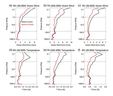
**Fig. 15.** RMS vector wind errors on 1 December 2014 for (a) NH, (b) TR, and (c) SH and RMS temperature errors for the (d) NH, (e) TR, and (f) SH. Black (red) lines are for assimilation of noisy (perfect) radiance data. Horizontal dashed lines indicate vertical range of assimilated stratospheric observations. Note that the ranges of the horizontal axes for each panel varies based
