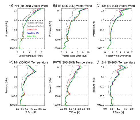
Fig. 18. RMS vector wind errors on 1 December 2014 for (a) NH, (b) TR, and (c) SH and RMS temperature errors for the (d) NH, (e) TR, and (f) SH. Colored lines are for ozone assimilation experiments with noisy radiance and ozone data with 2%
