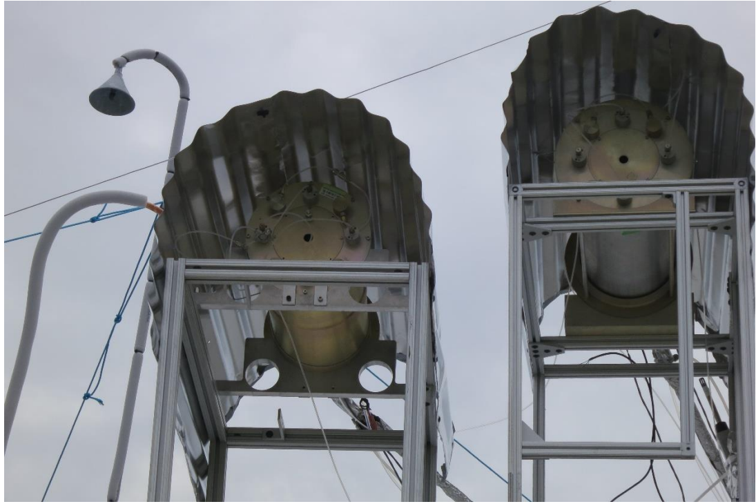
Fig. S1. Pictures of the OFRs operated at the T3 site.
