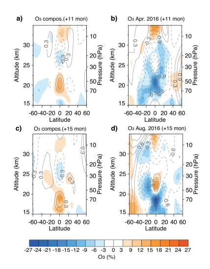
**Fig. 4.** Latitude-height cross sections of deseasonalized MLS ozone (filled) and temperature (gray contours) in the composite (a) 11 and (c) 15 months after the wind shear reversal based on 4 QBO cycles and during (b) April (+11 mon.) and (d) August 2016 (+15 mon.). Ozone and temperature values are shown in percent change from long term monthly averages with contour intervals every 3% and 0.3% respectively (zero contour is omitted).
