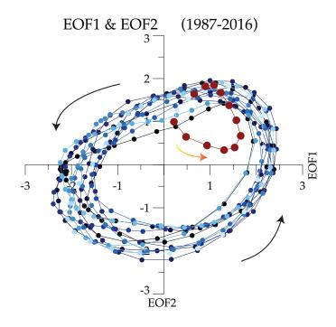
**Fig. 2.** Phase space diagram of the projection of the monthly equatorial zonal wind anomalies onto spacial structures EOF1 and EOF2. Time progression coincides with counterclockwise orbit transits. Dots represent each month from 1987-2016. Different shades of blue indicate different years from 1987-2015 (from darker to lighter) while red dots correspond to 2016.
