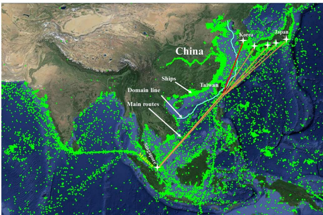
Fig. SI-1 Major shipping routes extracted from a real-time AIS digital map
