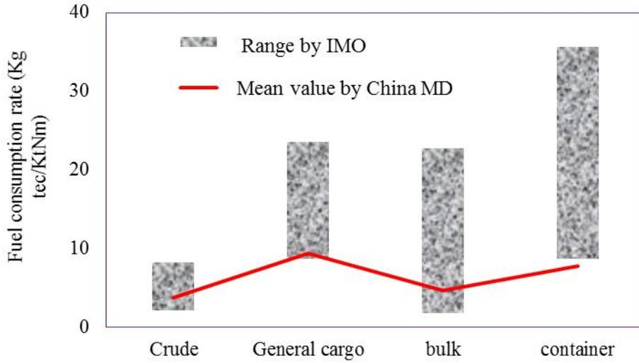
**Fig. SI-6 Range of fuel consumption rate used in this study**
