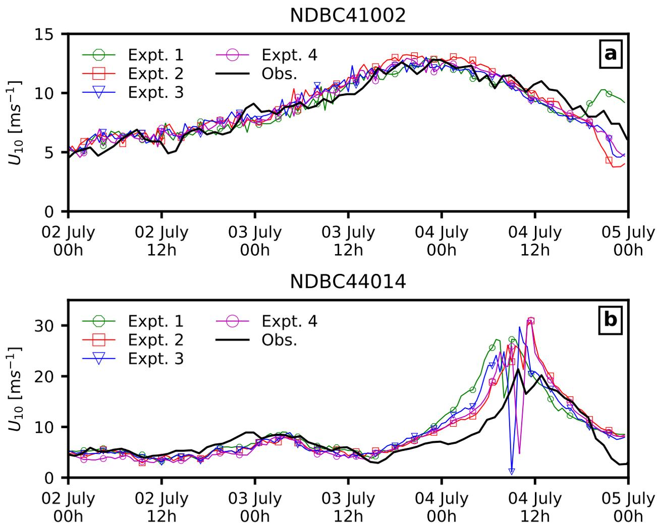
**Figure 7.** Comparison of coupled model results with NDBC buoys (a) 41002 and (b) 44014 for mean wind speed  $U_{10}$  [ms<sup>-1</sup>] at 10m elevation
