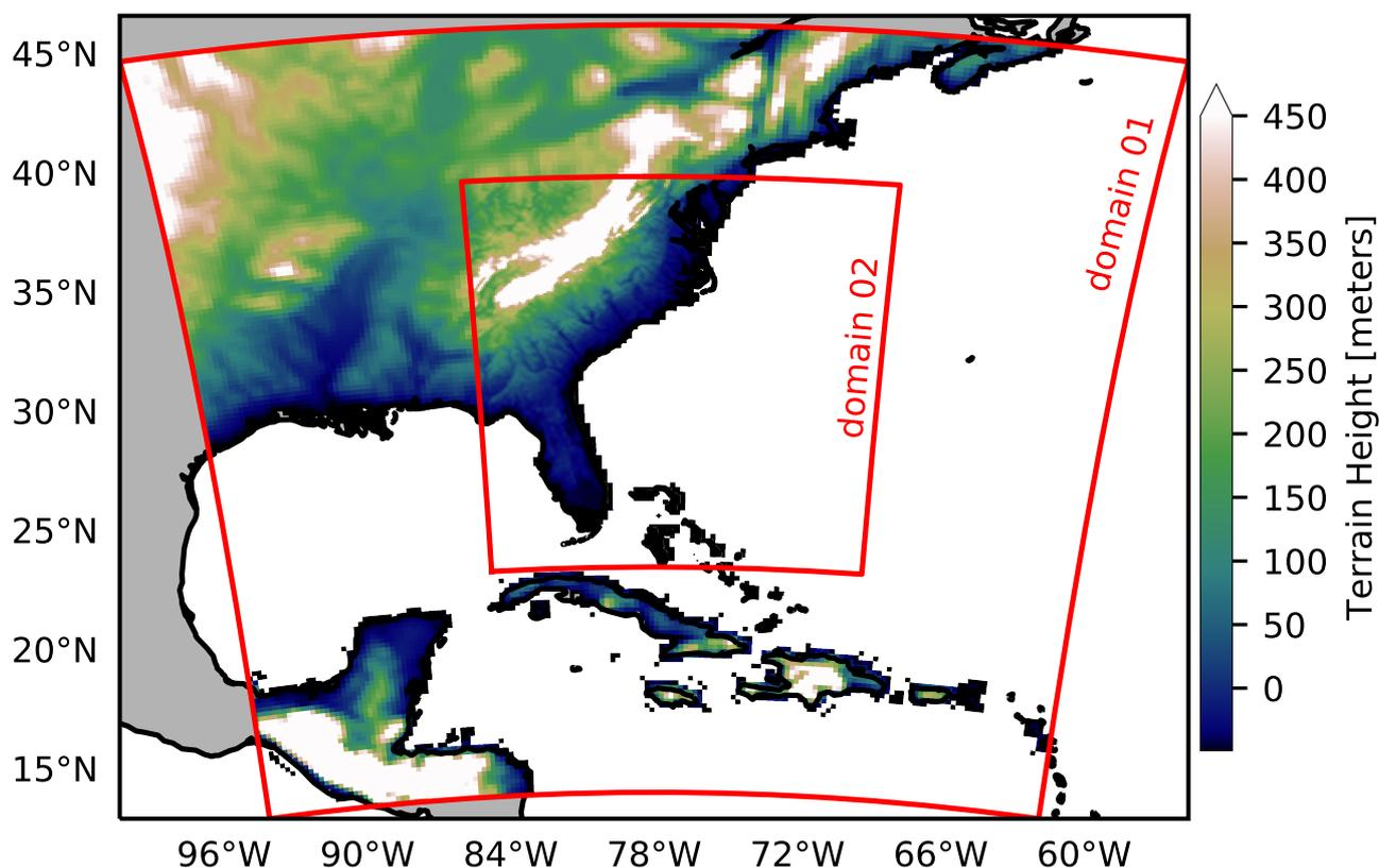
**Figure 1.** Horizontal extent and terrain elevation of atmosphere model domains in WRF, where horizontal resolution of outer domain is 21.6km while that of inner domain is 7.2km
