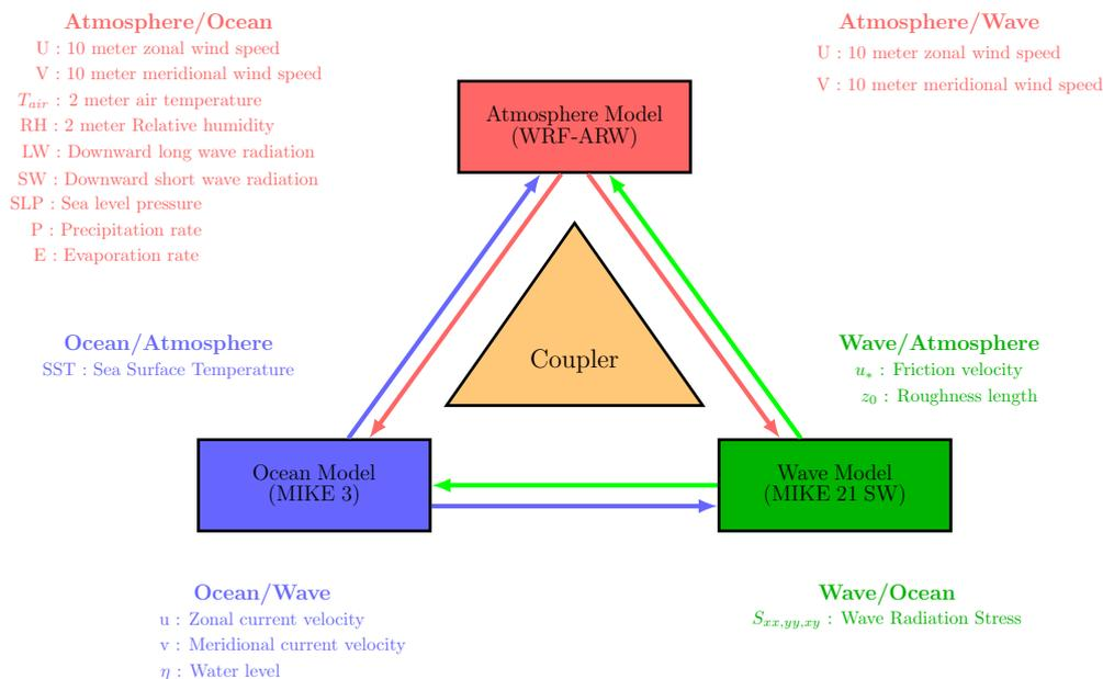
**Figure 3.** Schematics of coupled model components, where the atmosphere model (WRF), ocean model (MIKE 3) and wave model (MIKE 21 SW) interact through model coupling interface.
