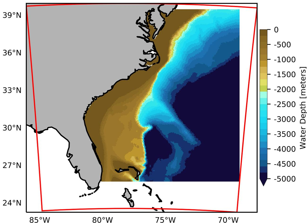
**Figure 2.** Horizontal extent and bathymetry of wave model domain in MIKE 21 SW together with the extent of inner domain used in atmospheric model (red)
