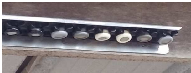
Figure 2: INDAAF passive samplers mounted in duplicate on a stainless steel holder.
