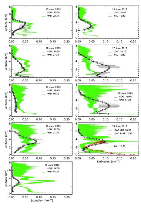
**Figure 8.** Comparison between LOAC extinctions and WALI lidar extinction at 350 nm. The LOAC error bars consider the uncertainty on the LOAC measurements and on the counting-extinction conversion; the WALI error bars are calculated from the individual measurement scatter.
