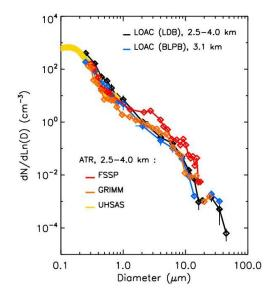
**Figure 11.** Comparison of the particle size distributions during the 16 June dust plume event over Minorca, obtained with LOAC instruments under balloons and particle counters on board the ATR-42 aircraft; measurement altitudes are given.
