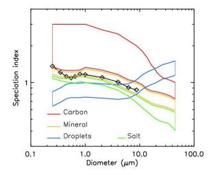
**Figure 2.** "Speciation zones" obtained in laboratory for several types of particles (color lines) and an example of LOAC speciation index obtained during ambient air measurements inside a Saharan dust plume at an altitude of 3.1 km (18 June 2013, 18:15 UT) above Minorca, Spain (diamonds).
