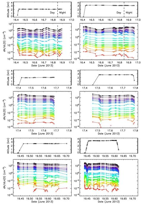
**Figure 13.** Flight altitude (up) and time evolution (bottom) of the LOAC-derived aerosol concentration for the 19 size classes, from BLPB flights from Minorca towards French coast. Colour coding is as in Fig. 6. Day-night transitions are indicated when appropriate.
