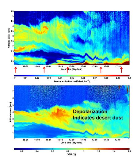
**Figure 5.** Lidar-derived time-height cross-sections of the aerosol extinction (top) and volume depolarization ratio (bottom) at Minorca from June 15, 22:00 to 17, 24:00 UT. The red arrows indicate the time of the 5 LDB launches. Courtesy of P. Chazette and J. Totems, after Chazette et al. (2016).
