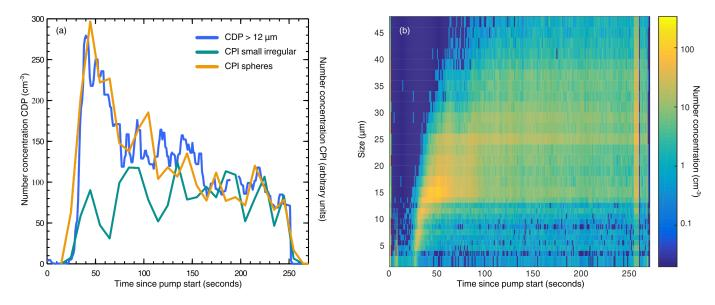
**Figure 2.** a) Measurements from the CPI instrument for the two particle habit classifications observed, small irregular (ice), green line, and spheres (drops), orange line, and the CDP for particles with sizes greater than 12  $\mu$ m, blue line. CPI data is shown without units because the data is qualitative. b) Size distribution of cloud particles measured by the CDP in MICC during an expansion experiment.
