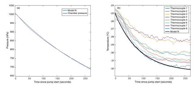
**Figure 1.** Example fits for pressure and temperature during an expansion experiment. a) The purple line is the pressure measured in the chamber by a Keller pressure sensor. The blue line is the pressure as simulated by ACPIM. b) Coloured lines show the temperature inside the chamber measured by 8 different thermocouples spread throughout the height of the chamber. The black line is the temperature as simulated by ACPIM.
