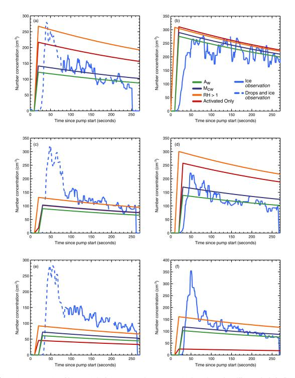
Figure 3. Number concentration of ice crystals in 6 chamber experiments and model simulations using different criteria for freezing. The solid blue line is the number concentration of ice measured in the chamber, dashed blue line represents the sum of liquid droplets and ice crystals initially formed and the other coloured lines are simulated ice number concentrations using different criteria for freezing in the model.
