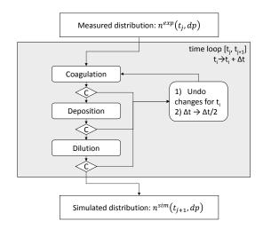
**Figure 7.** Flow diagram of the aerosol dynamics model calculating the changes to a particle size distribution  $n_{exp}(t_j, d_p)$  within the time interval  $[t_j, t_{j+1}]$ . *C* stands for control parameter and *t* stands for time.
