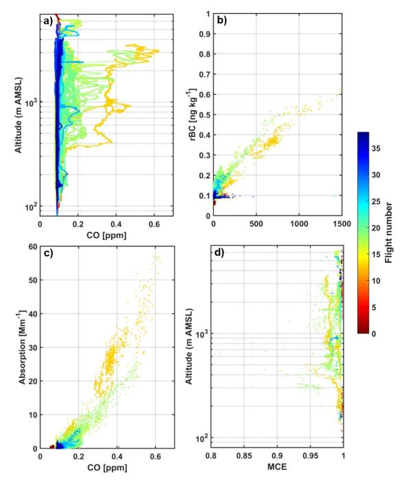
Figure 7. a) Vertical profile of CO concentrations, b) correlation between CO and rBC mass, and c) correlation between CO and absorption coefficient at 550 nm for each flight during the entire ACME-V campaign. Also shown is the calculated modified combustion efficiency (MCE) for data points classified as being impacted by the fires. All 1-second data are coloured by flight number.
