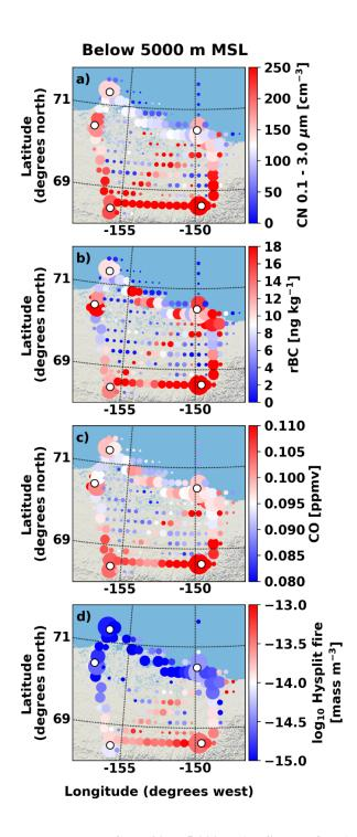
Figure 6. Same as Figure 2, but column averaged from 20 to 5,000 m AMSL and for a) CN with  $D_p = 0.1 - 3 \mu m$ , b) rBC mass, c) CO, and d) HYSPLIT aerosol mass concentrations with the five fire locations as the simulation start points.
