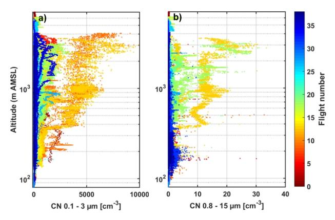
Figure 9. Vertical profiles of particle number concentrations measured from the a) CN with  $D_p = 0.1 - 3 \, \mu \text{m}$  and b) CN with  $D_p = 0.8 - 15 \, \mu \text{m}$  colored by flight number. Data shown are 1-second.
