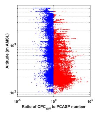
Figure 4. Ratio of the number concentrations of particles 3-10 nm in diameter CPC<sub>diff</sub> to PCASP number concentrations within 50 km of Deadhorse Airport. Blue indicates a ratio < 1 (i.e., PCASP > CPC<sub>diff</sub>) and red indicates a ratio > 1 (i.e., PCASP < CPC<sub>diff</sub>).
