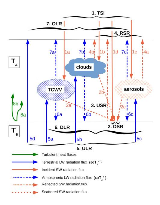
**Figure 1.** Simplified schematic of major processes controlling broadband radiation fluxes in the Sahel. Red arrows indicate shortwave radiation fluxes, blue arrows longwave radiation fluxes. For detailed description of arrows, please see section 2.1.
