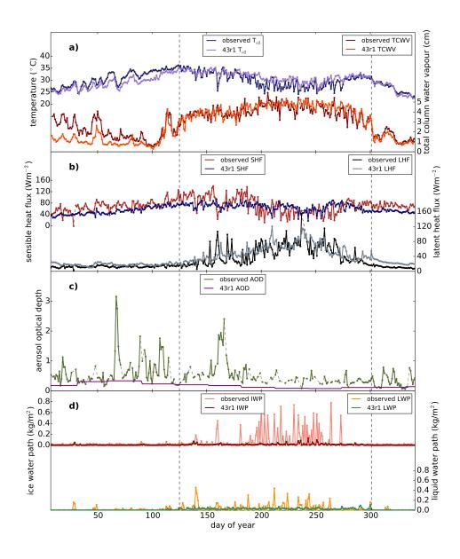
**Figure 4.** Observed and 43r1 non-radiative fluxes for Niamey during 2006. Plot (a) shows temperature and TCWV; plot (b) sensible and latent heat fluxes; plot (c) aerosol optical depth; and plot (d) ice water path and liquid water path. Dashed sections indicate imputed data, and dashed vertical lines indicate the beginning and end of the wet season.
