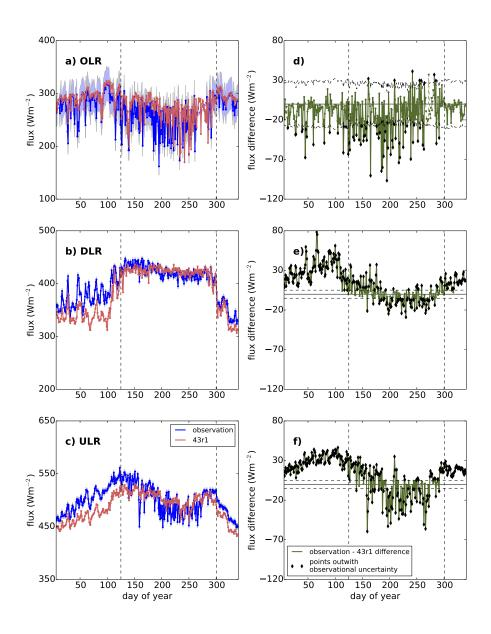
**Figure 3.** As Figure 2 but for longwave fluxes. Plots show observed and 43r1 (a) TOA outgoing longwave; (b) surface downwelling longwave; (c) surface upwelling longwave radiation fluxes; and the observation - 43r1 difference of these same fluxes in (d)-(f) respectively.
