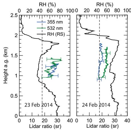
**Figure 11.** 2h mean profiles of the lidar ratio for the 23 February (left, 500 m vertical smoothing) and the 24 February 2014 (right, 750 m vertical smoothing). 532 (green line) without overlap correction, full overlap at 800–1000 m; 355 (blue line) with overlap correction. The RH profile of the radiosonde (black line) indicates the different layers.
