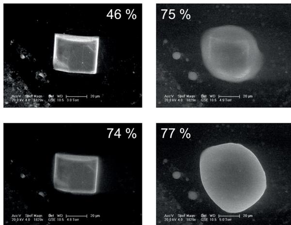
**Figure 1.** Sodium chloride deliquescence at 75% RH observed at laboratory conditions (at 4.9°C) in an environmental SEM (Scanning Electron Microscope). The dry cubic particle with sharp edges at RH of 46% becomes surrounded by a liquid sphere when RH increases to 77%.
