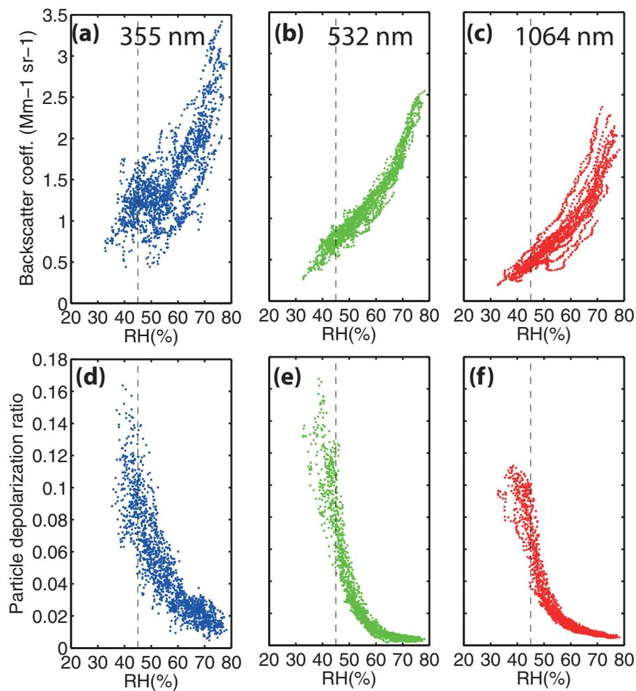
**Figure 12.** Correlation of the particle backscatter coefficient (top, a-c) and particle linear depolarization ratio (bottom, d-f) with RH for the three wavelengths 355, 532, and 1064 nm. The BERTHA measurement of 23 February 2014, 23:38–01:08 UTC, 375–1100 m height, are used (5 min temporal and 50 m vertical resolution). The dashed line marks the sea salt efflorescence point (45% RH).
