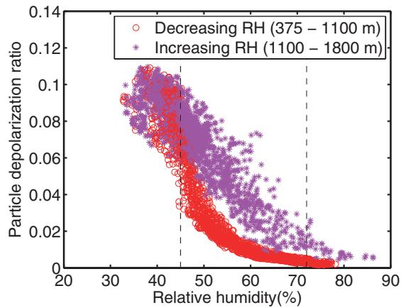
**Figure 13.** Correlation of the PLDR at 1064 nm and RH for the same settings as in Fig. 12, but for a different height interval (375–1800 m). Above 1100 m (purple stars) RH is increasing again, up to 80%, as can be seen in Fig. 9. The depolarization ratio decreases with increasing RH, but keeps higher values. The hysteresis effect between crystallization (45–48% RH, dashed line) and deliquescence (70–74% RH, dashed line) can be seen.
