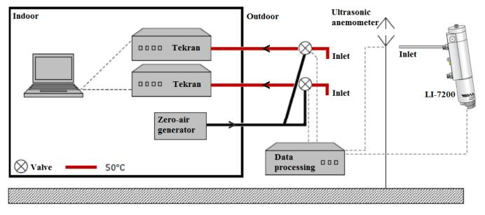
Figure 5: A Schematic representation of the GEM REA system.
