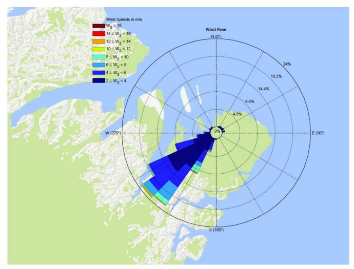
Figure 2: Wind rose centered at Villum Research Station, Station Nord. Length of the bars indicate frequency of the direction and color indicate the wind speed. Units in  $m \ s^{-1}$ .
