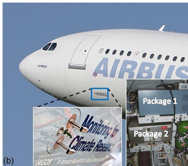
Figure 1: a) Schematic scheme of the temperature sensor attached to the humidity sensor mounted in the Rosemount housing (Helten et al., 1998). b) Packages 1 and 2 installed aboard the AIRBUS A340-300, and the inlet plate including the Rosemount housing (photograph by courtesy of Lufthansa).
