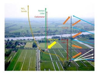
Figure 19: Schematic layout of the CINDI-2 campaign superimposed on an aerial picture of the CESAR site. Main instrument classes are indicated. The NO<sub>2</sub>-sondes were launched from close to the tower. A long-path DOAS was placed at a distance of about 4 km from the tower that was able to scan several retro-reflectors at different altitude levels.
