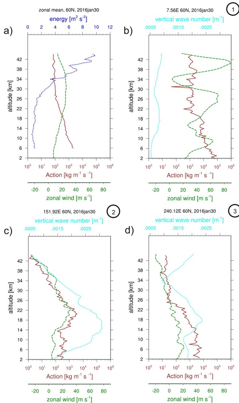
**Figure 5.** Vertical profiles at 60°N, 30 January 2016. Zonal mean (a) of kinematic wave energy (dotted, blue), wave action (solid, red) and zonal wind (dashed, green). Local vertical profiles at 7.56°E (b), 151.92°E (c) and 240.12°E (d) with the vertical wave number (dotted, light blue), wave action (solid, red) and zonal wind (dashed, green). Local profiles according to markers of Fig. 4.
