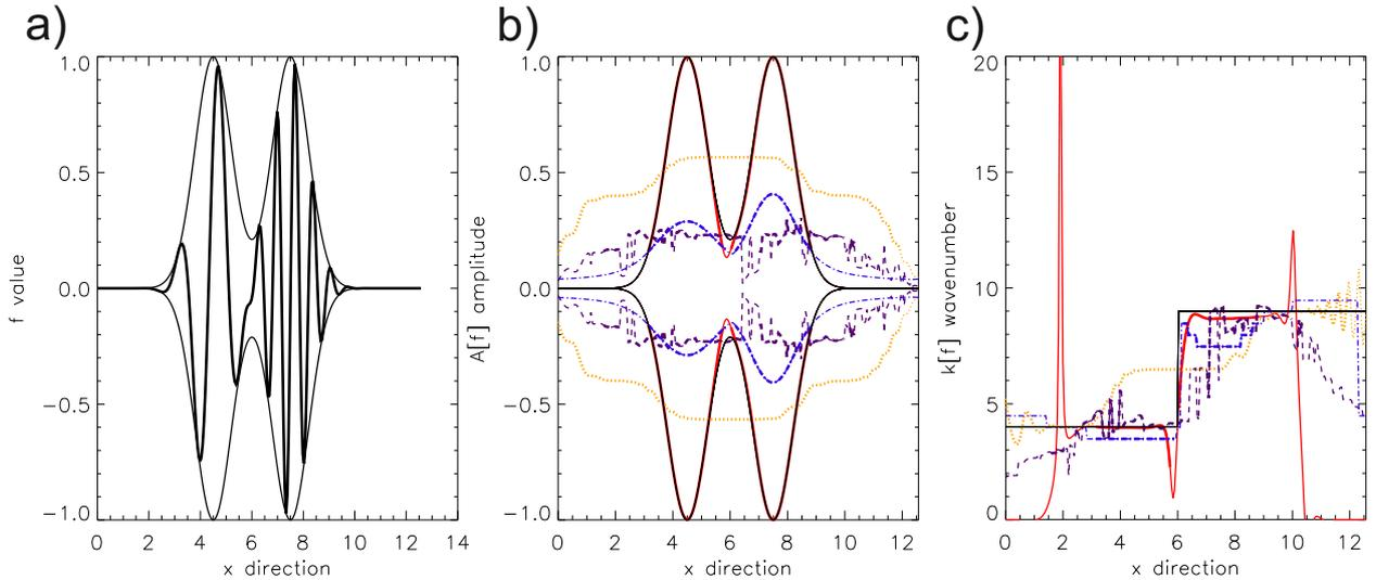
**Figure 1.** One-dimensional test function (bold line, left figure) adapted from Zimin et al. (2003) and its envelope. Comparison of amplitude (centre) and wave number (right) calculated by different methods: UWaDi (solid, red), DIV (dotted, orange), S-3D (dashed, violet) and 3D-ST (dash-dotted, blue). Valid estimates are drawn in bold.
