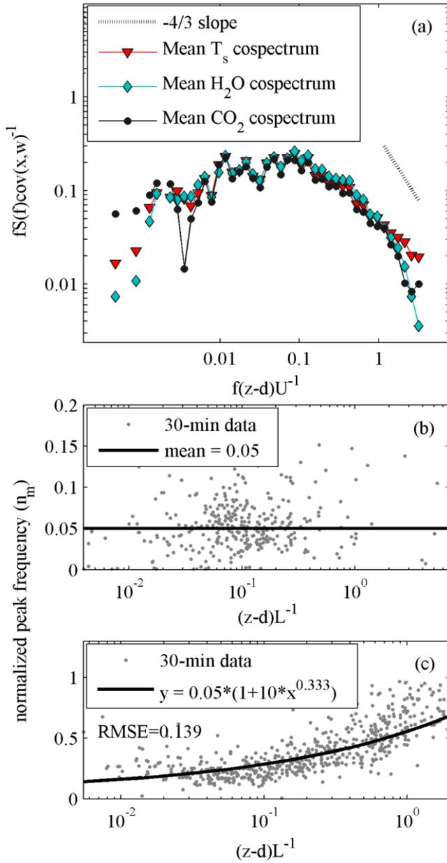
**Figure 2:** (a) Normalized frequency-weighted co-spectra of temperature, carbon dioxide and water vapour as a function of normalized frequency measured on 16 July 2015, 11:00-13:30 (mean value of stability parameter  $(z-d)L^{-1} = -0.023$ ). The two following subplots show the 30 min values of the normalized peak frequency  $n_m$  versus the stability parameter  $(z-d)/L$  in unstable condition (b) and stable conditions (c).
