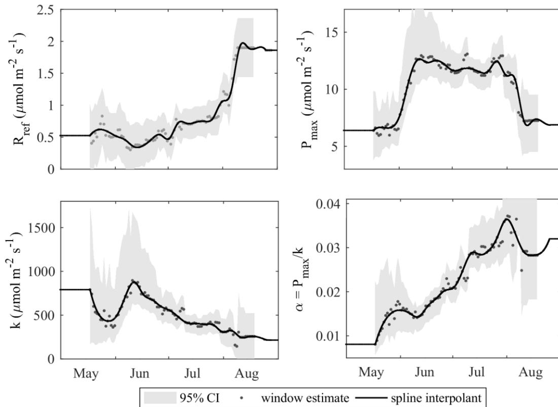
**Figure 7:** time series of the CO<sub>2</sub> flux model parameters. The dots are the daily values evaluated in a moving time window, and the solid line is a spline-interpolant, while the shaded area shows the 95% confidence interval, which is calculated at each time window step. The interpolated parameter lines stretch to the beginning of May and end of August, showing the constant values used on the edges of the study period.
