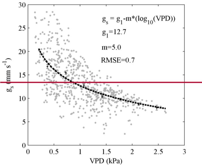
**Figure 11:** Surface conductance versus vapor pressure deficit demonstrating a well known relationship. The grey dots are the 30 min average data, black dots with error bars the bin averages, and the dashed line the fit (the function is specified in the insert).
