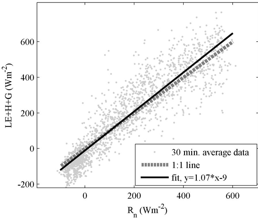
1085 **Figure 67:** Energy balance plot. The sum of latent and sensible heat fluxes and soil heat flux is plotted against net radiation flux. A linear function is fit to the data and shown together with a 1:1 line. The mean ratio of  $(LE+H+G)$  to  $R_n$  is 0.99.
