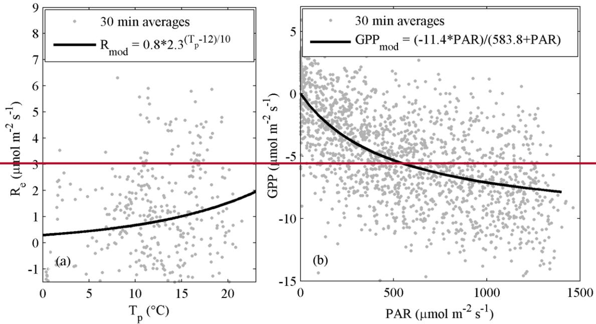
**Figure 3** CO<sub>2</sub> flux : (a) Night time ecosystem respiration as a function of peat temperature at 5 cm depth; (b) average light response function fit to all available data.
